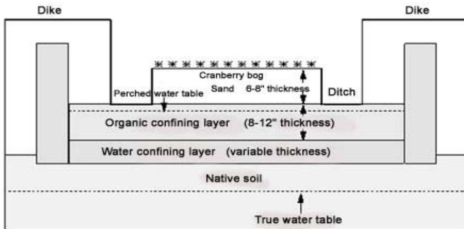
**Figure 1. Cross-section showing construction of cranberry bog with location of organic and water confining layers in system using perched water table design.**
