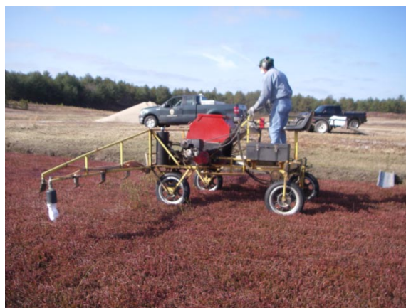
Gephardt drop spreader delivering granular herbicide to the cranberry farm surface. Note white droplet of foam at left, which helps to guide the driver.
