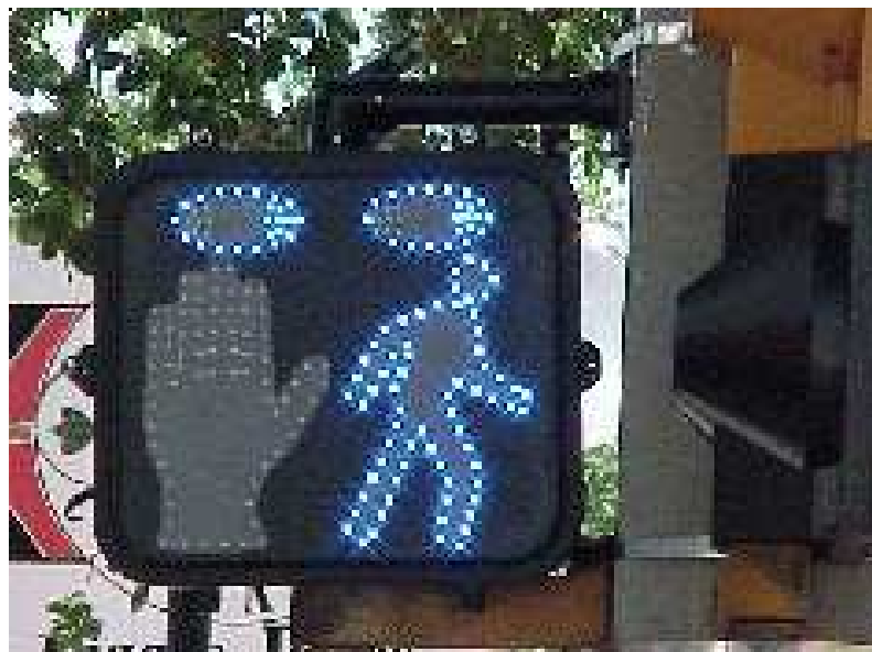
Figure 8 Animated LED “Eyes” Pedestrian Signal in Clearwater, FL (18).
