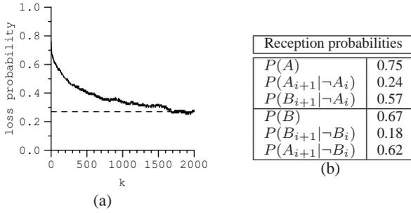
**Figure 6: (a) Probability of losing packet  $i+k$  from a BS to vehicle in VanLAN given that packet  $i$  was lost. (b) Unconditional and conditional packet reception probability from two BSes to the vehicle.**
