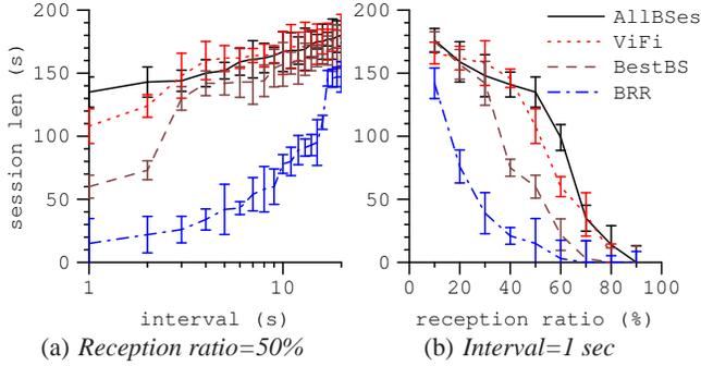
**Figure 7: The median session length in VanLAN as a function of the reception ratio threshold and time interval used to define adequate connectivity. The curves for *AllBSes* and *BestBS* are identical to those in Figure 4.**
