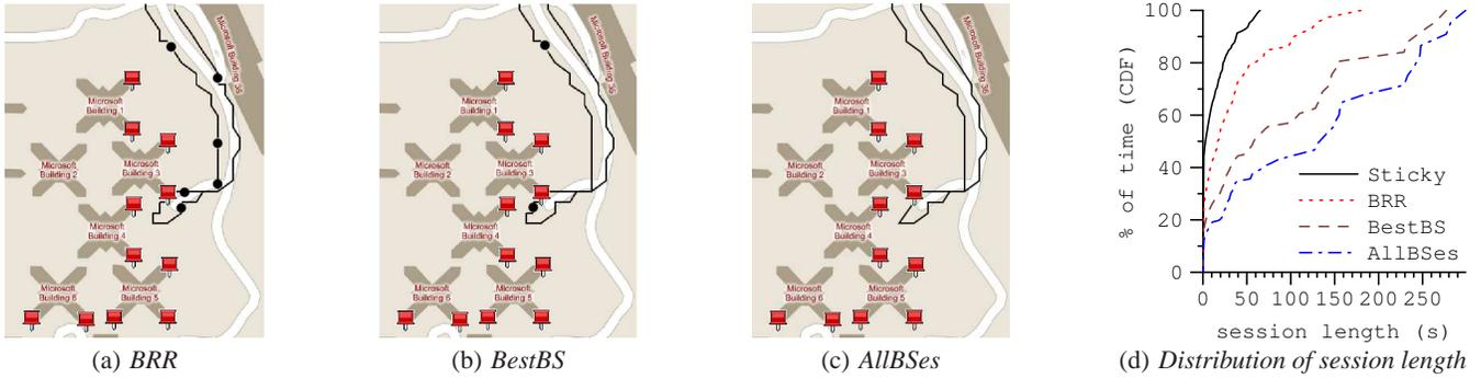
**Figure 3:** (a)-(c): The behavior of three handoff methods for an example path segment in VanLAN. Black lines represent regions of adequate connectivity, i.e., more than 50% reception ratio in a one-second interval. Dark circles represent interruptions in connectivity. (d): The CDF of the time the client spends in a session of a given length.
