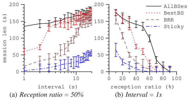
**Figure 4:** The median session length in VanLAN as a function of the time interval (a) and the minimum reception ratio (b) used to define adequate connectivity. The left graph has logarithmic  $x$ -axis. Error bars represent 95% confidence intervals.
