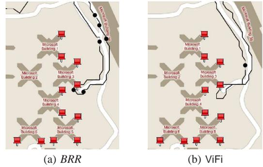
**Figure 8: The behavior of *BRR* and ViFi along a path segment in VanLAN. Black lines represent regions where the reception ratio was more than 50% in 1-second intervals. Dark circles represent interruptions.**
