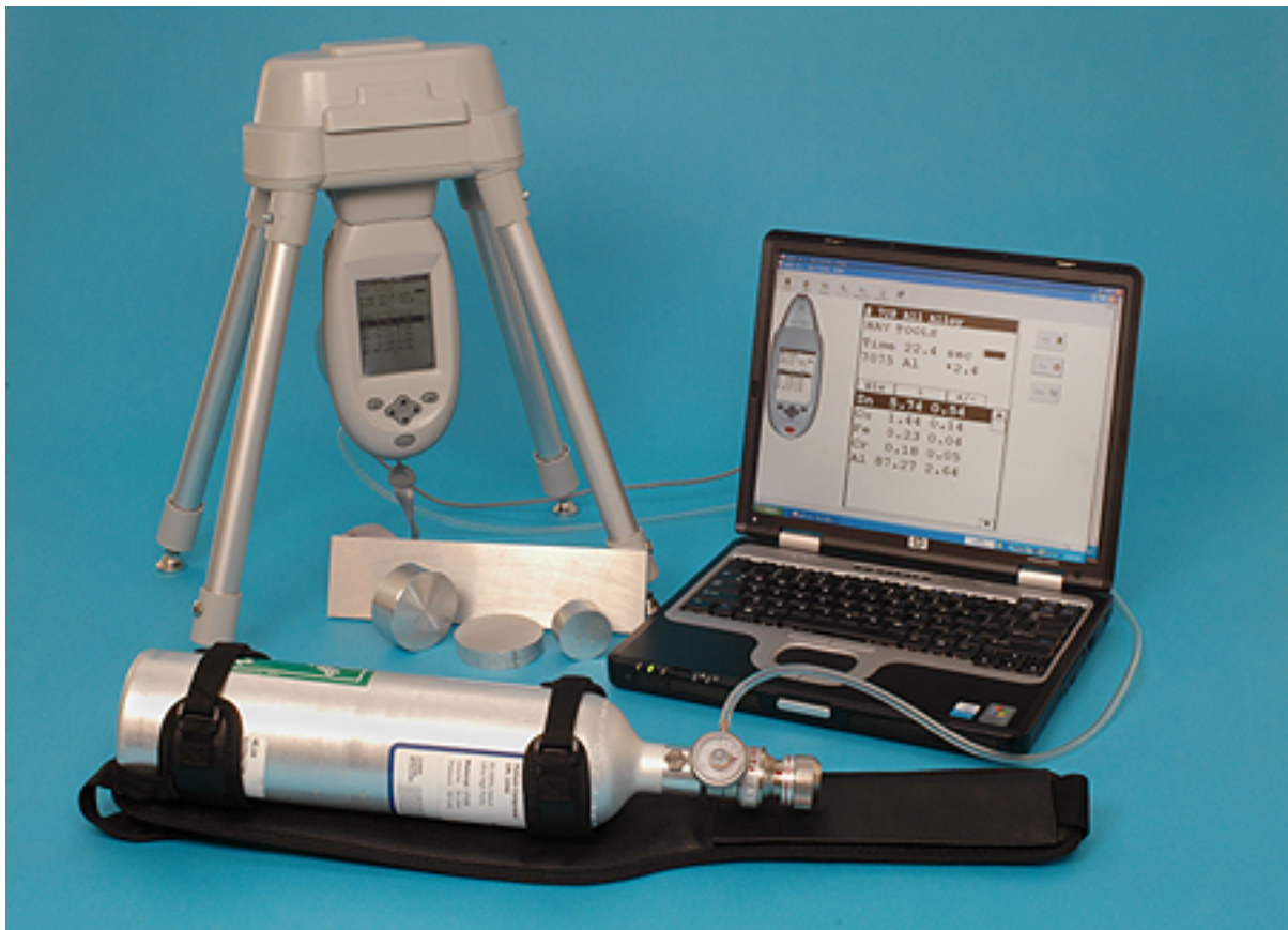
Figure 1. The Niton XLt 500 He system with sample stand, analyzer, and Helium purge.
