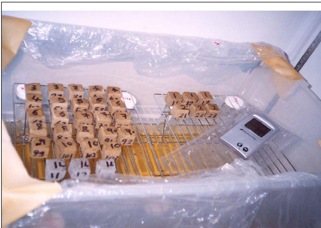
Figure 1. Tailings specimens inside the moisture chamber
