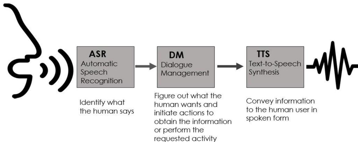
Figure 1 – Simplified block diagram of the technological components of SDS<sup>20</sup>
