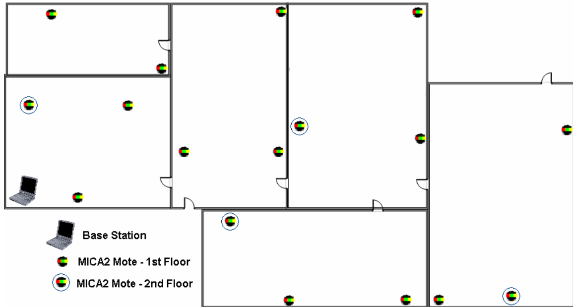
Figure 11: An approximate layout of the hardware experiment performed to verify software functionality. The test actually took places on two floors with this same room layout. The nodes that were on the second floor are depicted with circles.
