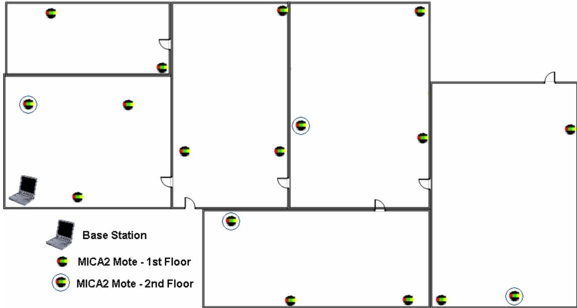
**Figure 11: An approximate layout of the hardware experiment performed to verify software functionality. The test actually took places on two floors with this same room layout. The nodes that were on the second floor are depicted with circles.**
