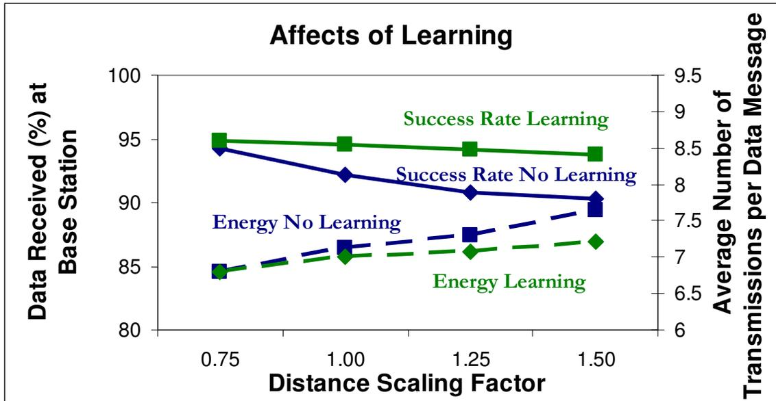
**Figure 17: Comparing the success rate and energy between using learning and not using learning. The solid lines represent success rates and align with the left hand axis, the dashed lines represent energy and align with the right axis.**
