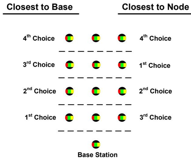
**Figure 9: The next best neighbor selection algorithms. The circled node is the one which is running the algorithm and each dashed line represents a depth increase in the routing tree. The rankings of nodes of a given depth with each selection algorithm is shown**
