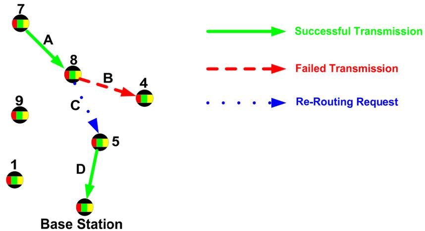
**Figure 7: An example of fault tolerant re-routing.**
