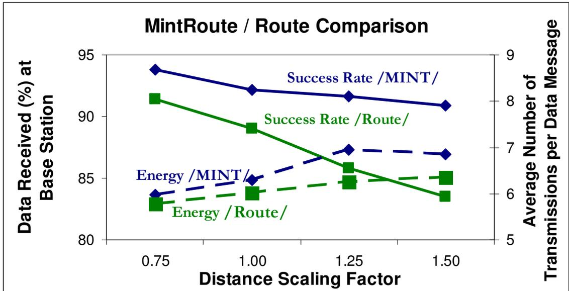
**Figure 32: Comparing between MINTRoute and Route.** On the left hand y-axis we see the percentage of data that is received at the base station. The two plots which have solid lines align with this axis. On the right hand side is a measure for energy, the two plots with dashed lines align with this axis.
