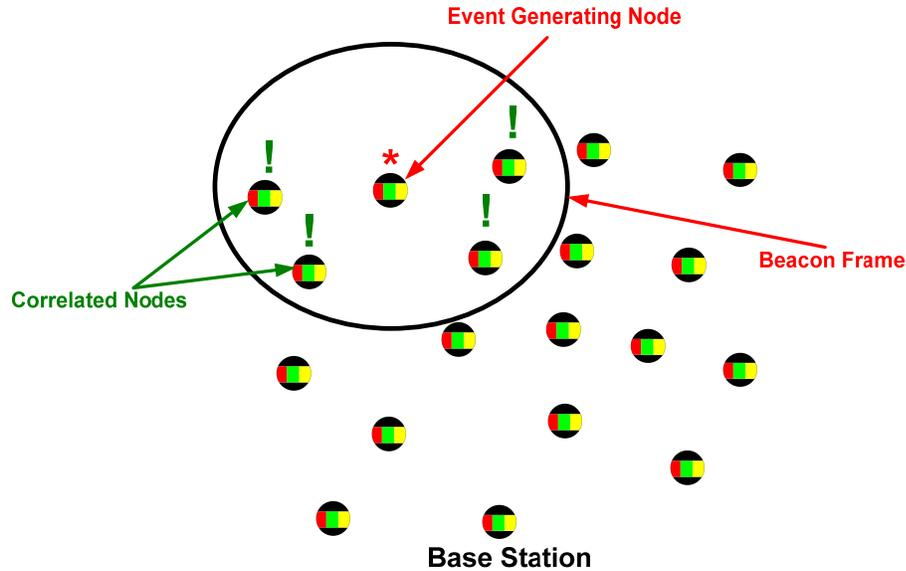
**Figure 20: The process for simulating correlated events. The starred node is the node that generates the event, the nodes with exclamation points check to see if they will generate a correlated event.**
