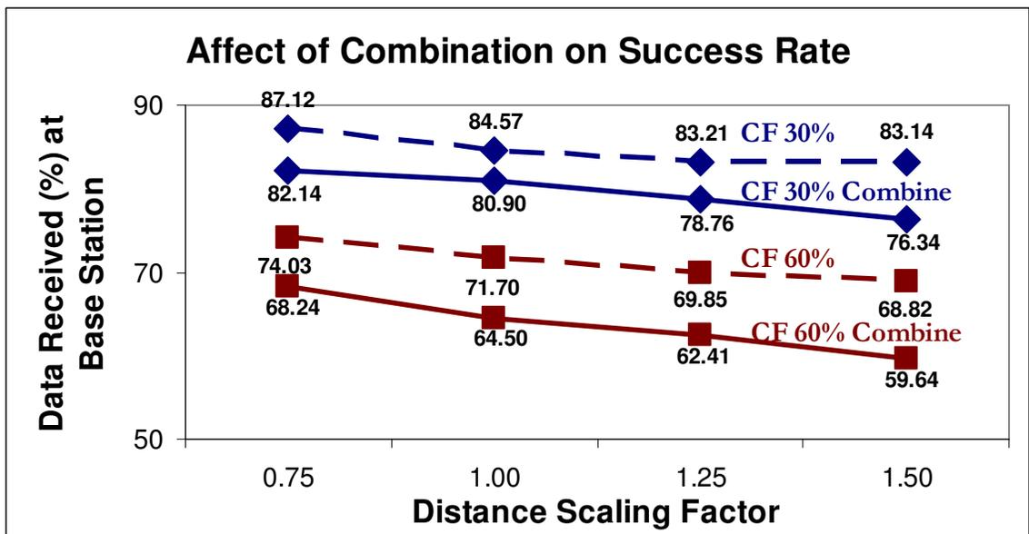
**Figure 24: The effects of the combining correlated messages on the success rate of messages in the network. The dashed lines represent the case of not combining and the solid lines represent what happens when we start combining.**
