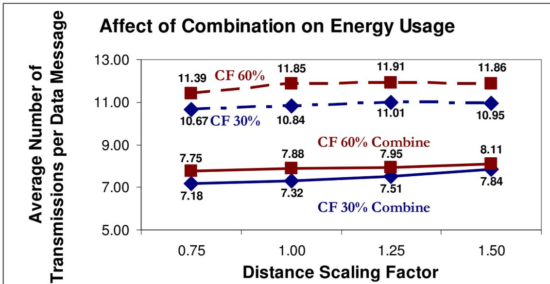
**Figure 25: The effects of combining correlated messages on the number of transmissions required for each original message. The dashed lines represent no combinations and the solid represents the case of combining similar messages.**
