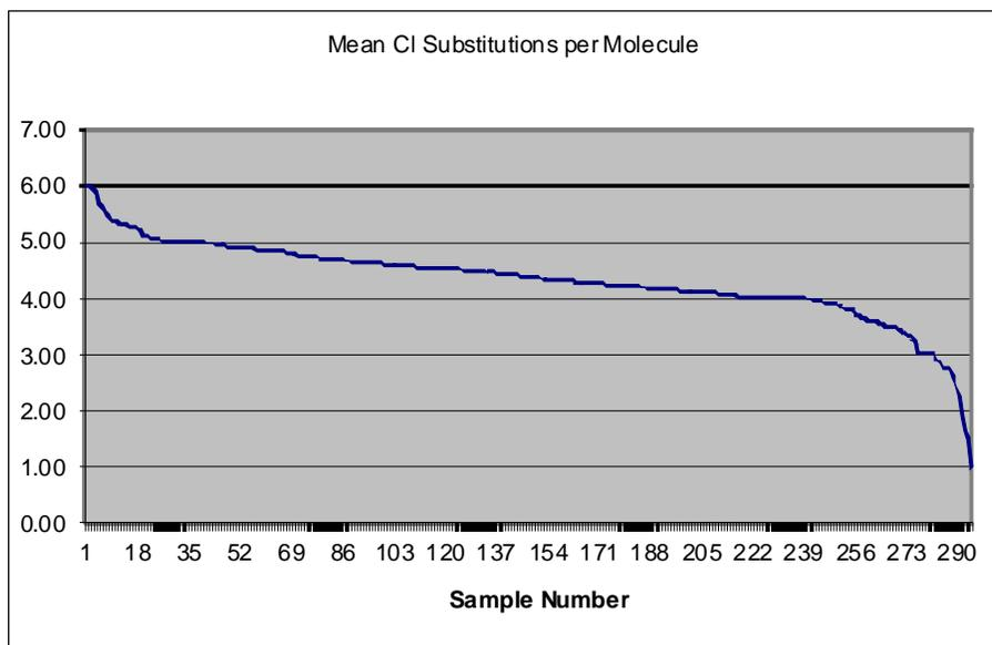
*Figure 2.* This chart shows the average chlorine substitutions per PCB molecule (along the y-axis) for the study sample set in descending order. Note one sample contained solely deca-chloro-biphenyl and that sample is not represented on the chart.
