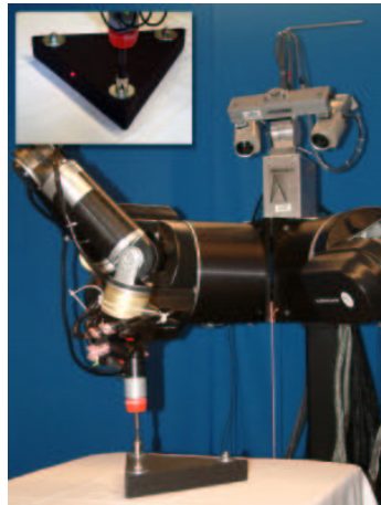
Fig. 1. The UMass Torso consists of an articulated, stereo biSight head, two 7-DOF Whole Arm Manipulators (WAMs), two 3-fingered hands (each finger is equipped with a six-axis force/torque sensor), and a quadraphonic audio input system.
