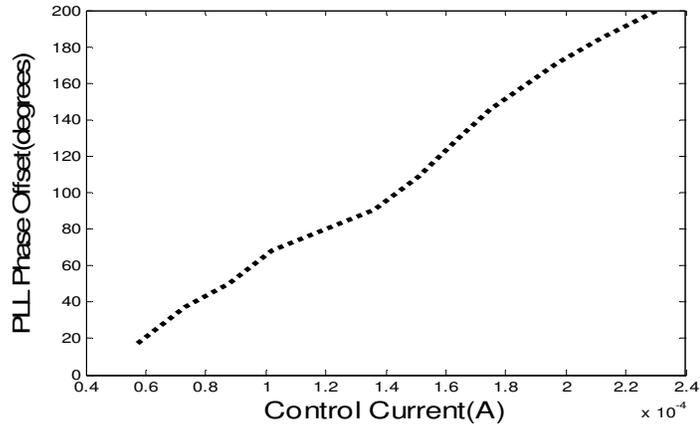
**Figure 31: CPLL output phase vs. Control current**
