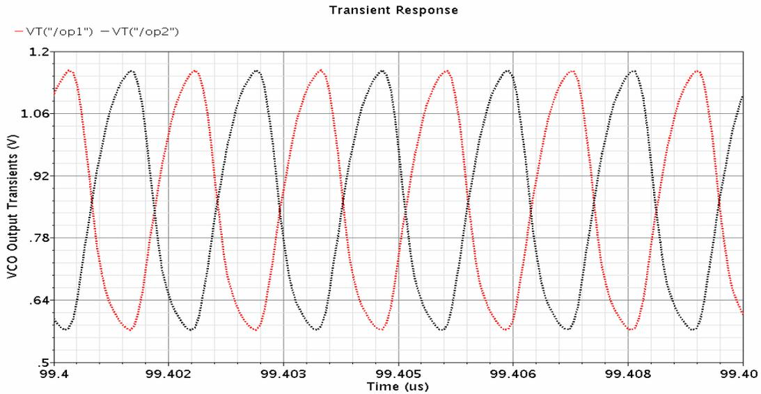
**Figure 77: CPLL VCO output waveforms at steady state**
