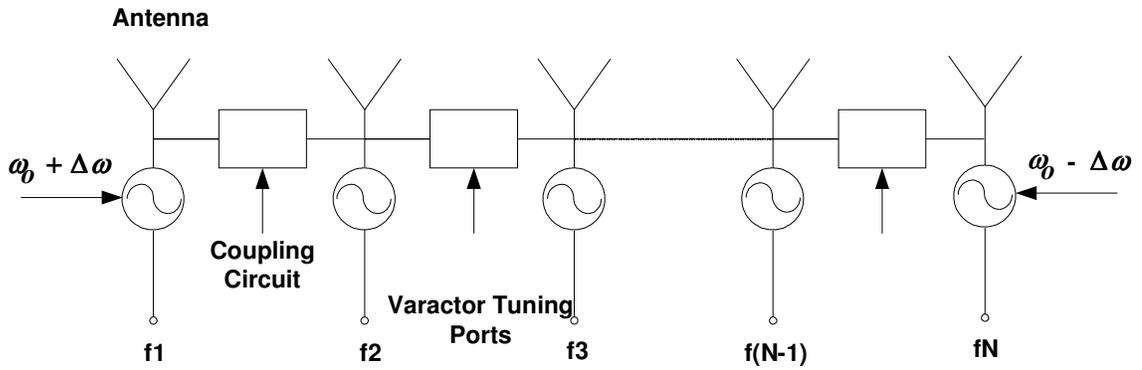
**Figure 2 : N-Oscillator system using bidirectional coupled Oscillators**
