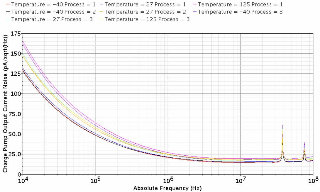
**Figure 53: Charge Pump Output Current Noise(A/sqrt(Hz))**
