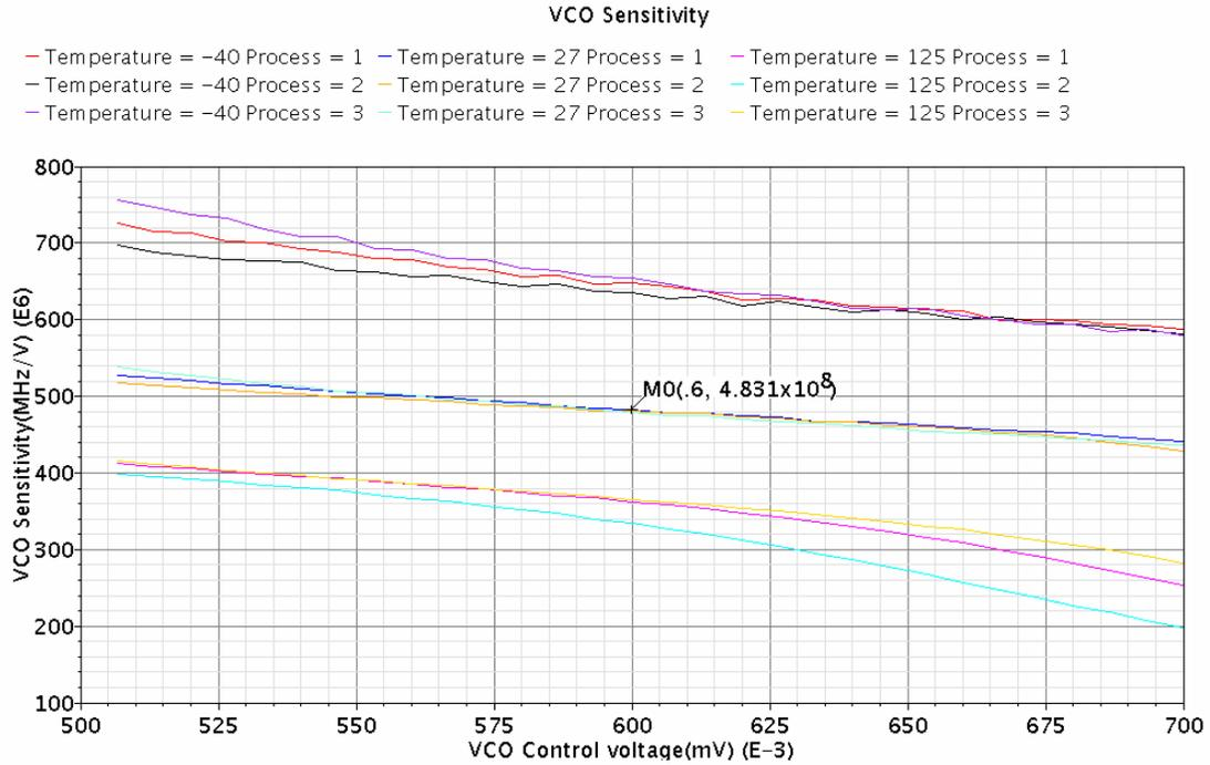
**Figure 63: VCO Sensitivity vs VCO control voltage**
