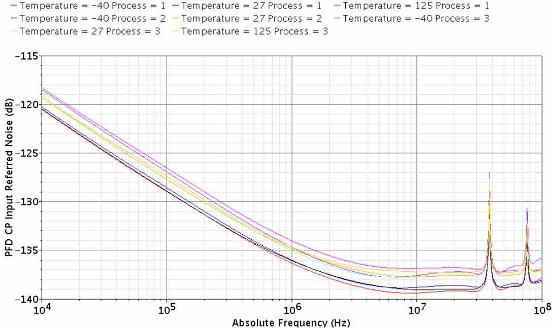
**Figure 54: PFD CP Input Referred Noise(dB)**
