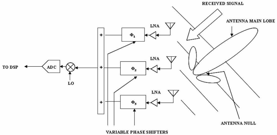
**Figure 3: Typical Phased Array Receiver**
