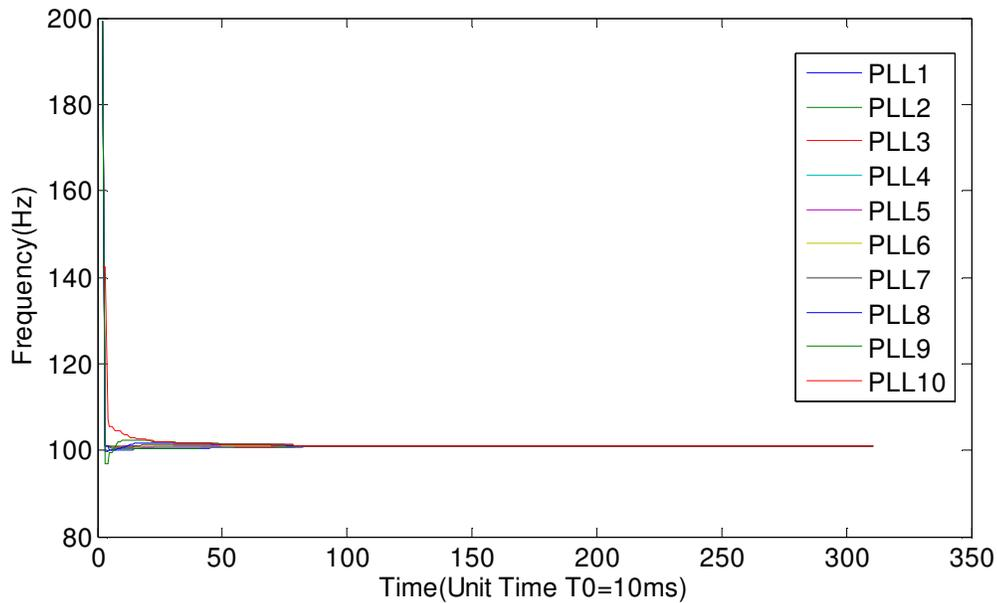
**Figure 8: N PLL system frequency convergence plot**
