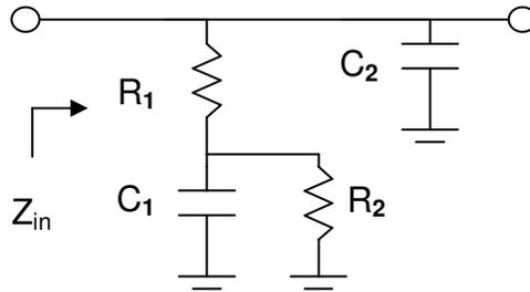
**Figure 11: Loop Filter Schematic**
