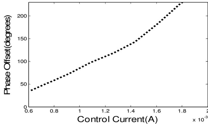
**Figure 28: CPLL output phase vs. Control current**
