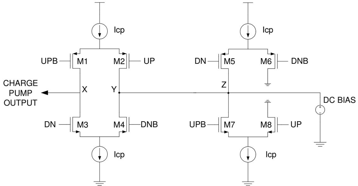
**Figure 48: Charge Pump Implementation Compatible with PFD CML**
