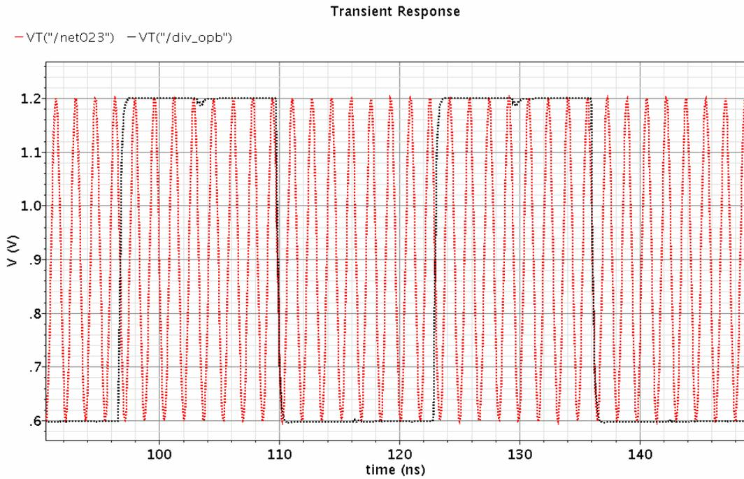
**Figure 73: Frequency Divider transient response**
