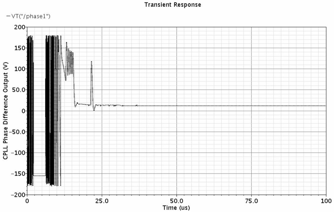
**Figure 76: CPLL Phase difference output transient**
