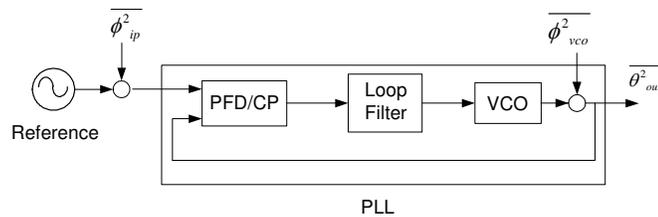
**Figure 20: Single PLL with different noise sources**
