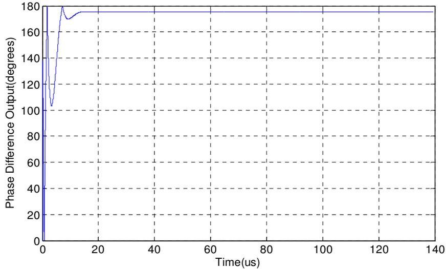
**Figure 35: Phase Difference Transient for the CPLL system**
