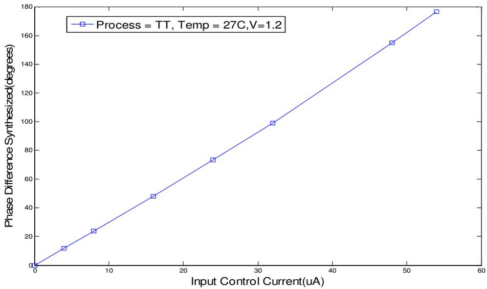
**Figure 80: CPLL Phase difference output vs control current**
