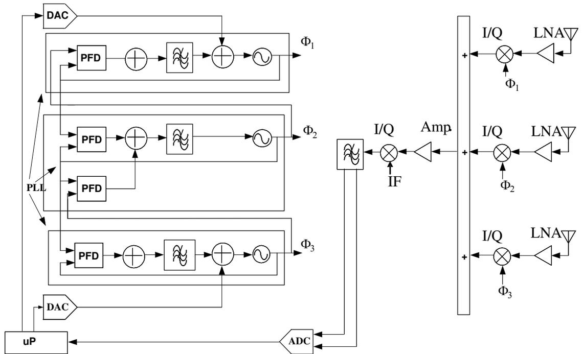
**Figure 4: Proposed Receiver Architecture without Phase Shifters**
