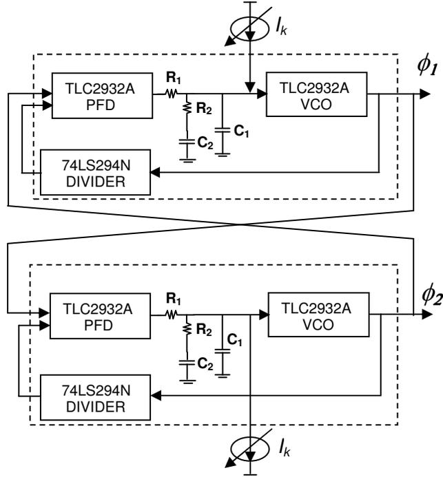
**Figure 30: Implemented Coupled PLL system with dividers**
