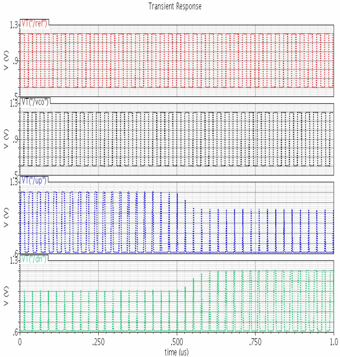
**Figure 47 : PFD Input and Output Waveforms**
