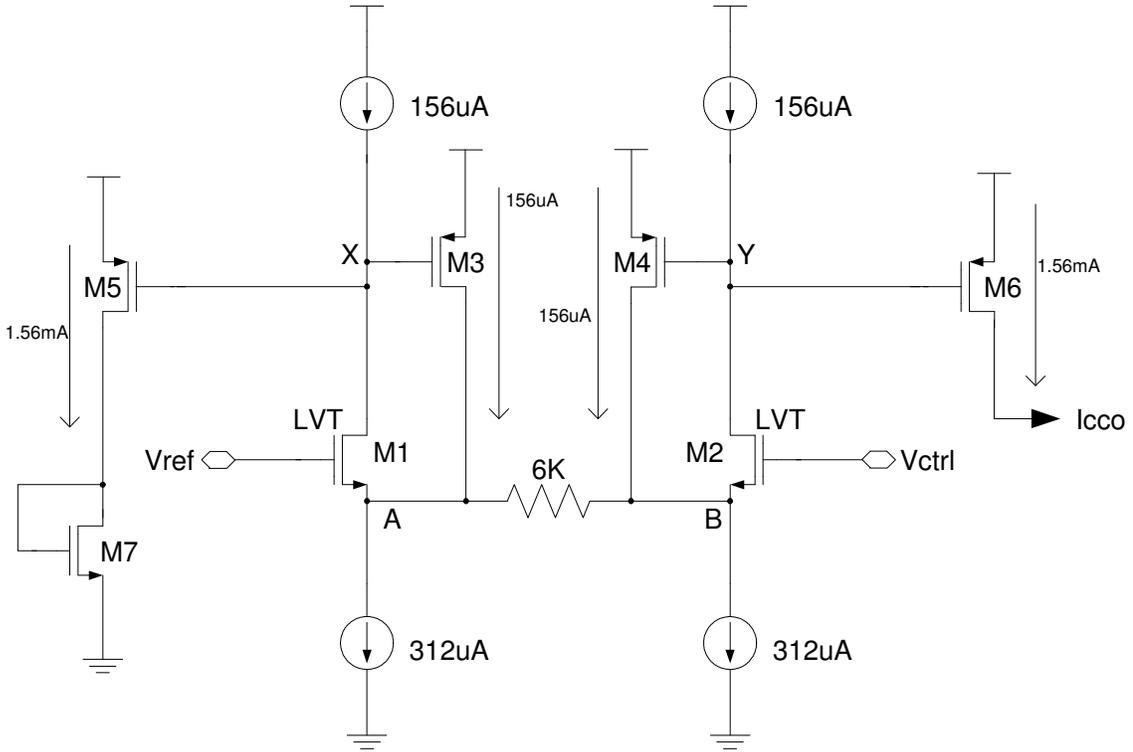
**Figure 56: Circuit Schematic for the V-2-I converter**
