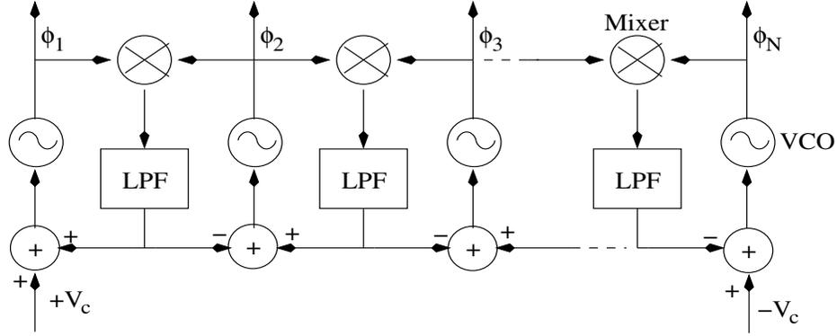
**Figure 1: N-PLL system using bidirectional coupled PLLs**
