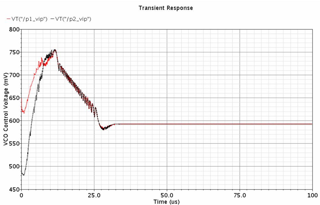
**Figure 75: CPLL VCO control voltage input transient response**
