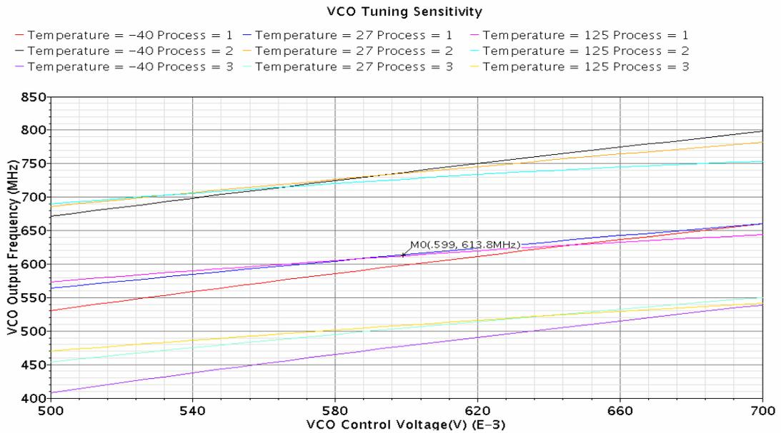
**Figure 62: VCO output frequency vs control voltage**
