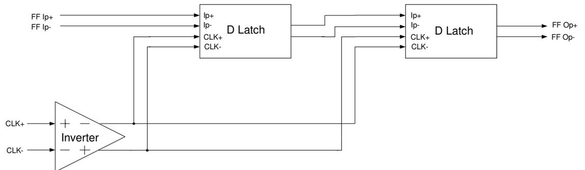
**Figure 69: Schematic of Master Slave D Flip Flop**
