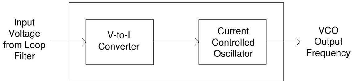
**Figure 55: System Block diagram for the VCO**
