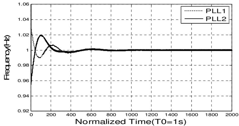
**Figure 18: Frequency Convergence for the Phase Frequency Synthesizer**
