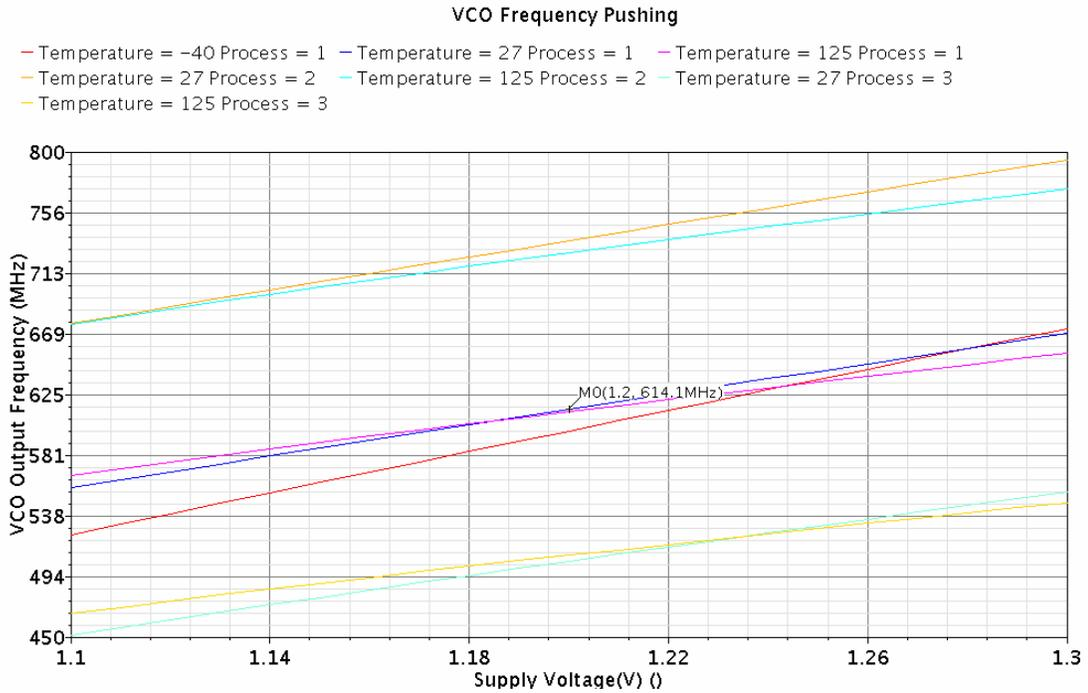
**Figure 64: Frequency Pushing**
