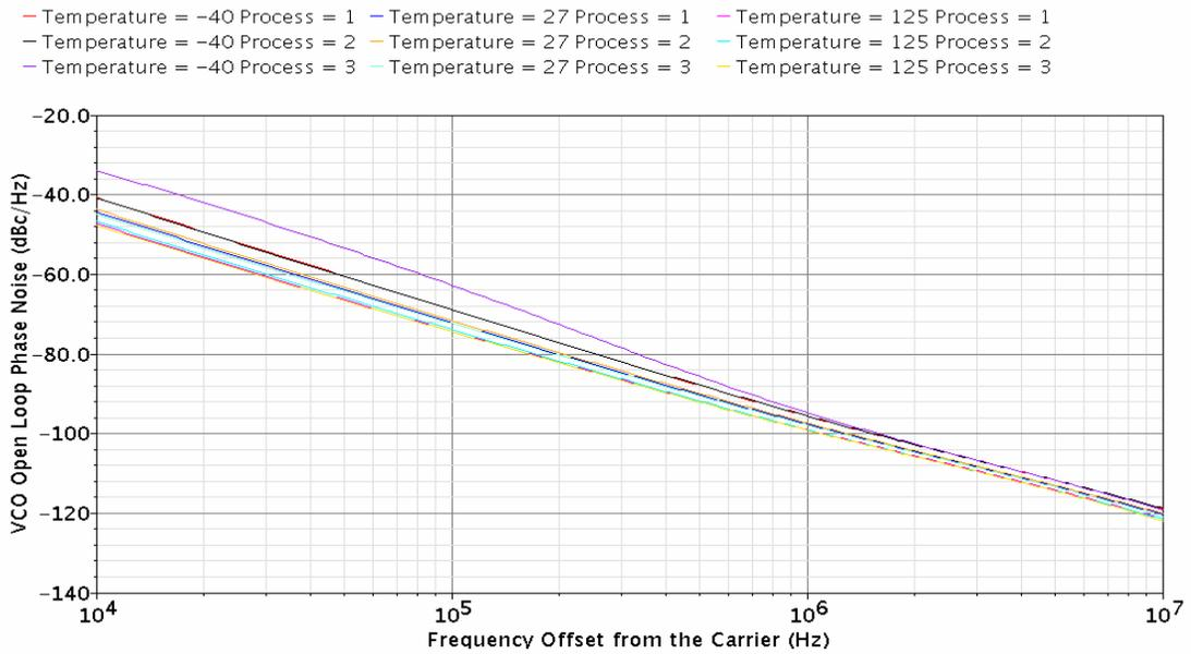
**Figure 61: VCO Open Loop Phase Noise**
