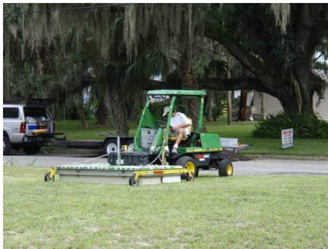
Figure 5. Radar tomography survey. Photograph by author.
