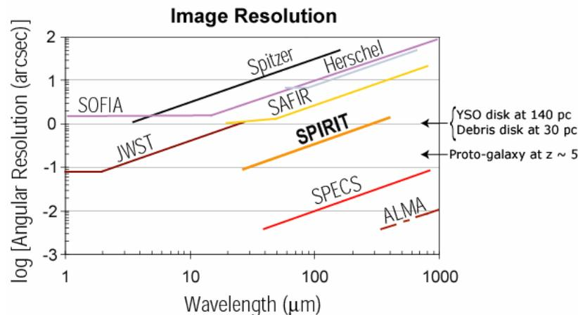
**Fig. 1** – Angular resolution available with current, next-generation, and future infrared and submillimeter observatories. SPIRIT will provide one hundred times better angular resolution than the Spitzer Space Telescope. The resolution is comparable to that of JWST, but at ten times longer wavelengths, where Young Stellar Objects (YSOs) emit most of their light.
