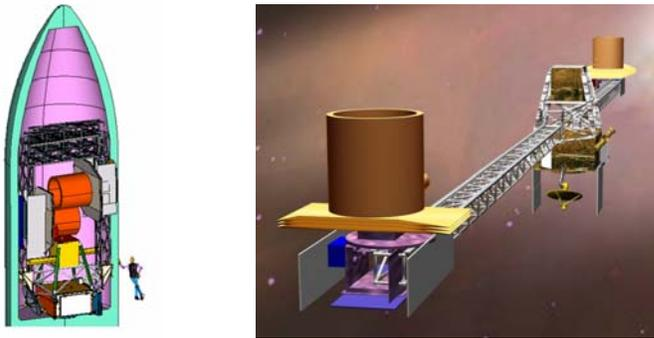
**Fig. 4** – SPIRIT and its expendable launch support structure, when stowed for launch (left), are 8.7 m tall and were designed to fit into an Atlas V 5-medium fairing. The deployed observatory is shown in an artist’s concept (right).
