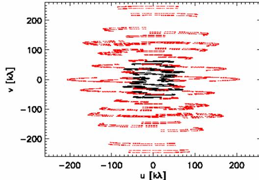
**Figure 1.** The  $u - v$  coverage for our high resolution interferometric imaging of AzTEC4 and AzTEC8 for both the compact (COM: black), and extended (EXT: red) configuration. For further details, including weather conditions and on-source integration times, see Table 1.
