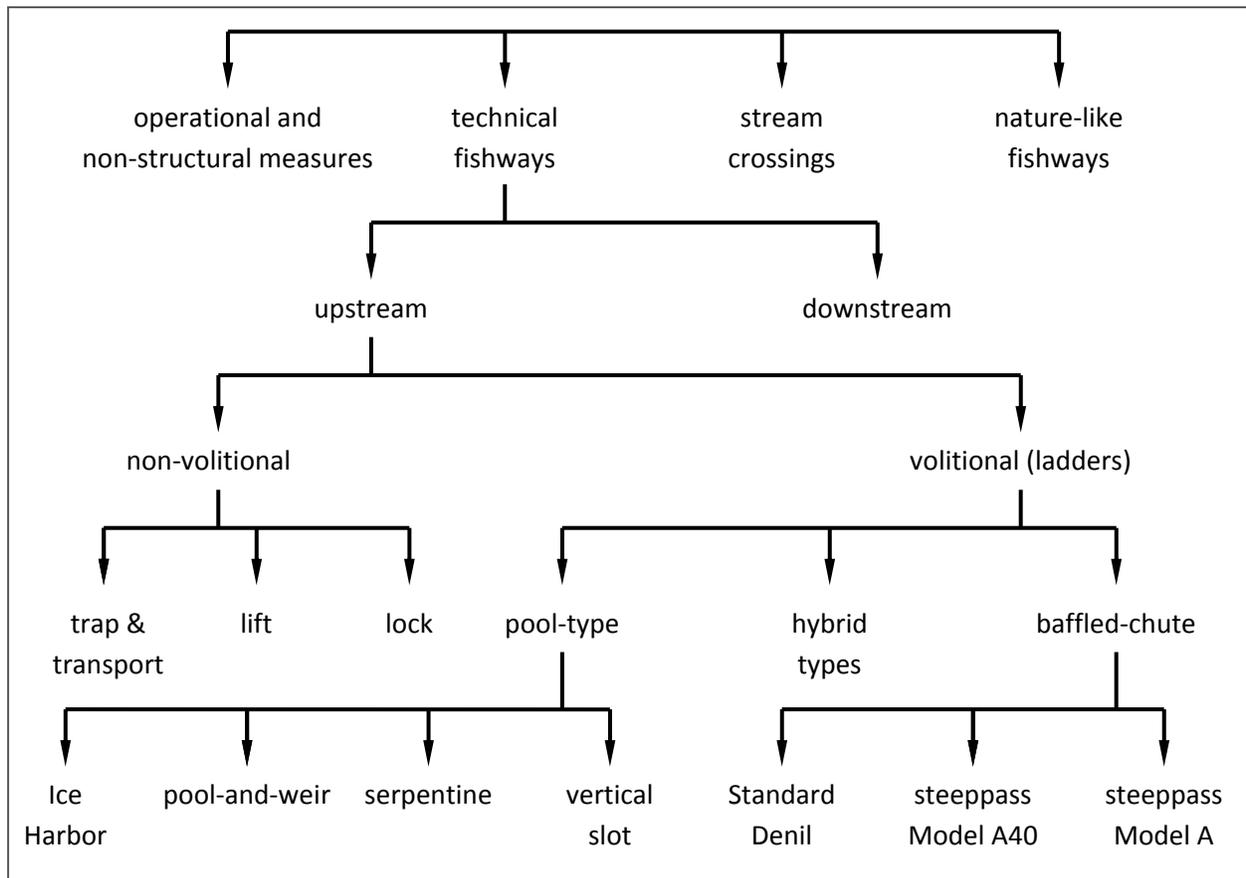
Figure 1. Common fishway types in the eastern U.S.
