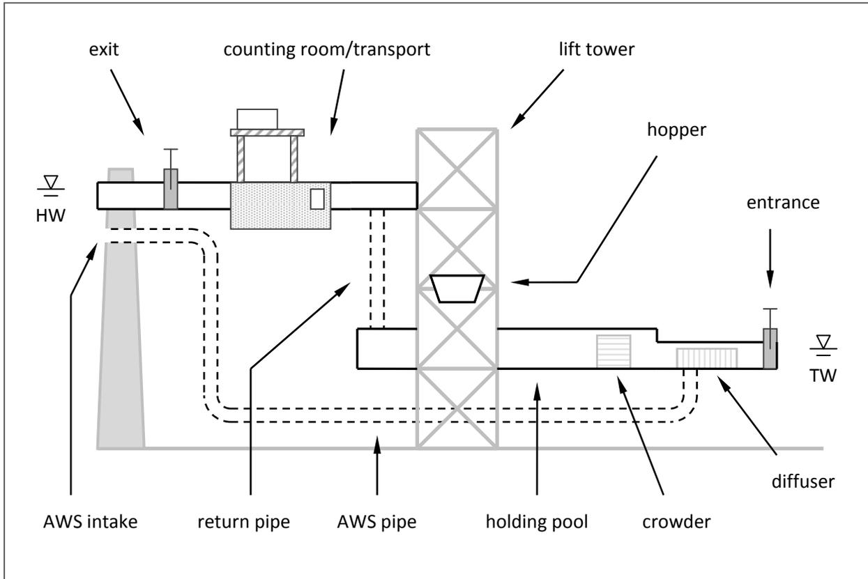
Figure 3. Major components in typical non-volitional fish lifts
