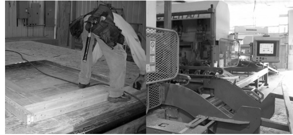
Fig. 1. Prefabricated panel operation of Ferrell and Barker (L) and computer controlled saw mill at Truss Manufacturing Company
