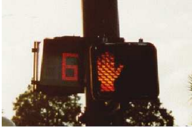
Figure 5 Countdown Signal in Lake Buena Vista, FL (17).
