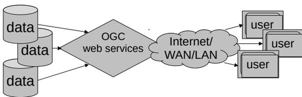
Figure 1: Internally managed data (or metadata) from multiple data stores are provided using OGC compliant (CSW, WFS, WMS, SOS) and other web services to the internet, enabling internal and external consumption, via both web and desktop clients.
