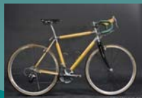
Laminated wood bike frame Sylvan Cycles
