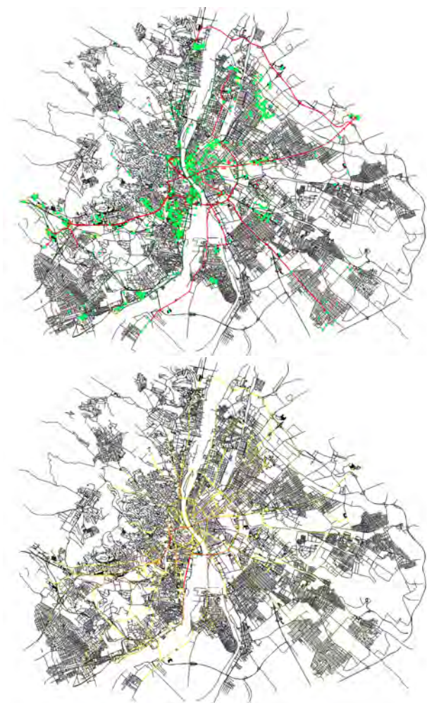
Figure 7: Visualization of the agent based traffic simulation: (a) Running agents; (b) Traffic congestion levels.
