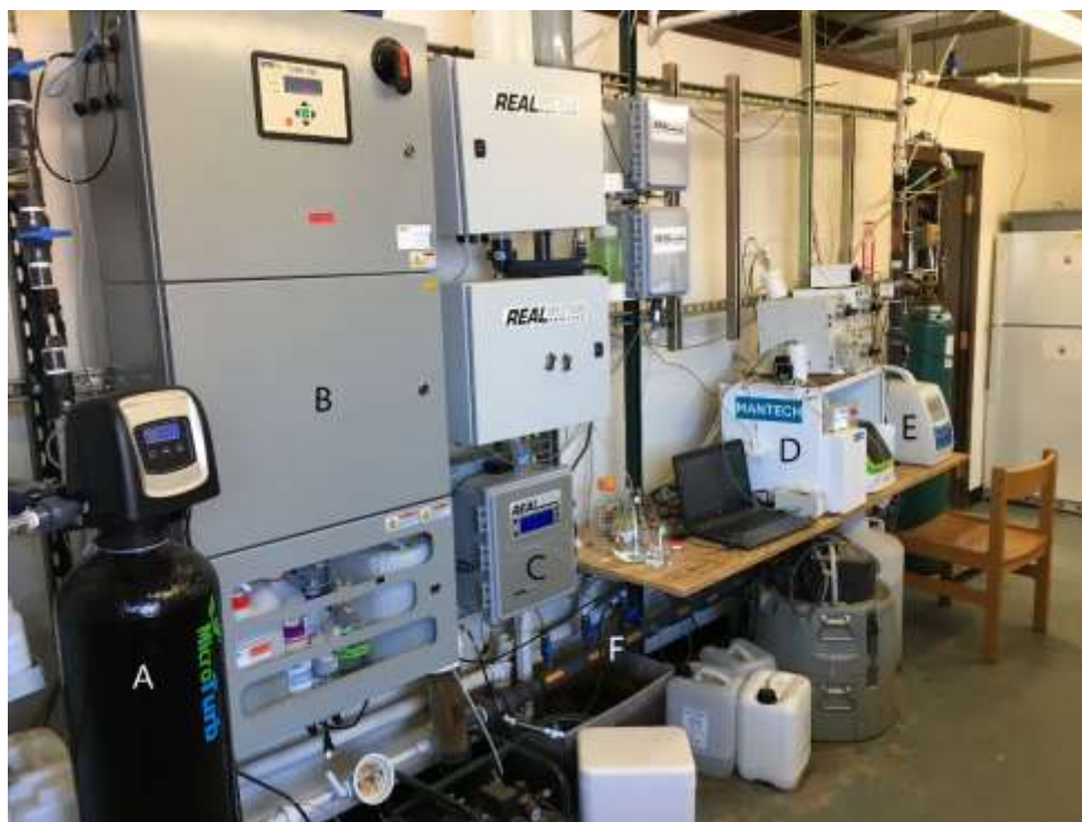
Figure 1. Experimental Setup: (A) – NextSand Microturb Filter; (B) – Aquametrology Systems THM-100; (C) – RealTech UV254; (D) – Mantech PeCOD (not enough available data); (E) – Suez GE Portable TOC Series M5310C; (F) – Water distribution manifold.
