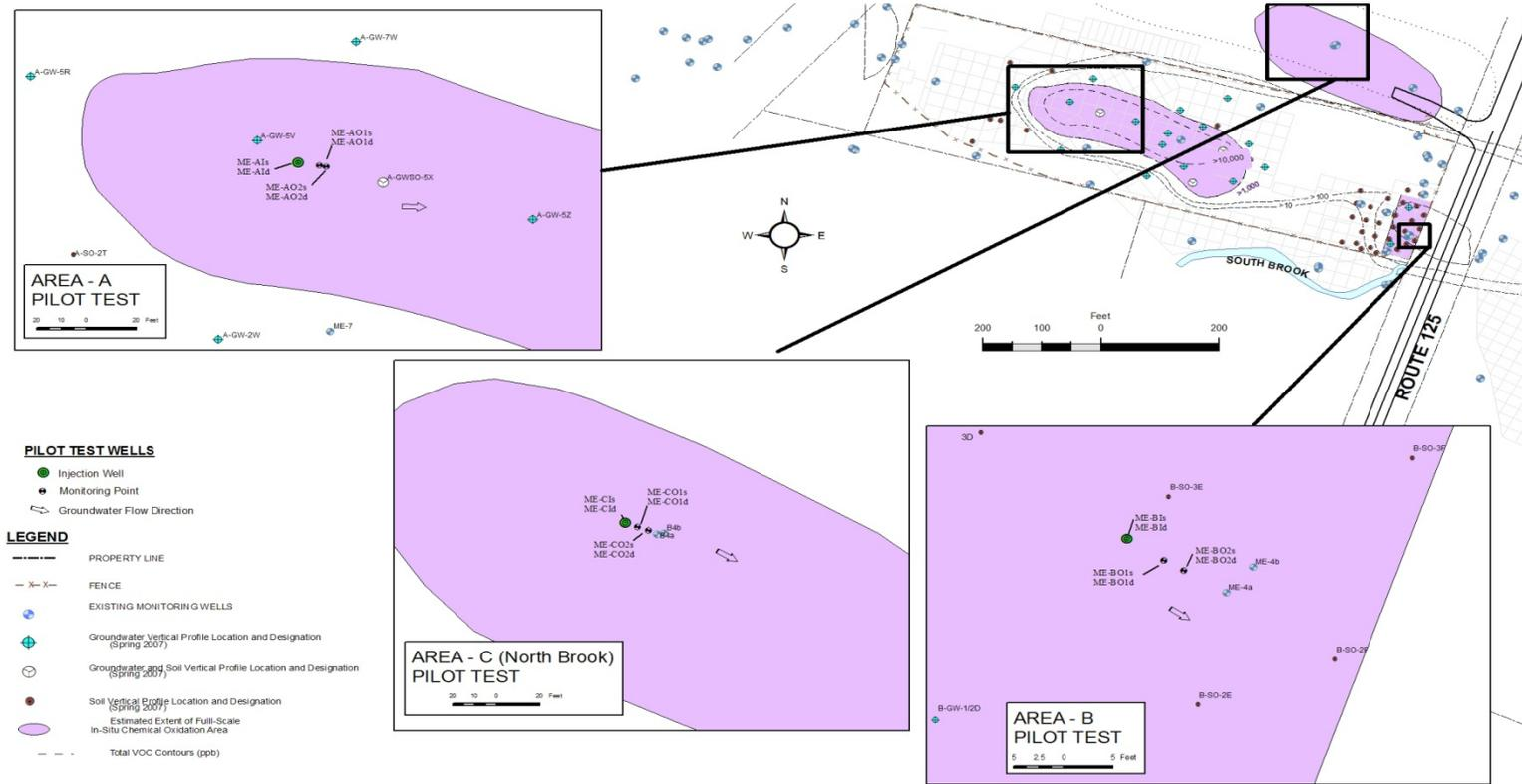
Figure 1. Site Map Showing Three Chemical Oxidation Pilot Test Areas
