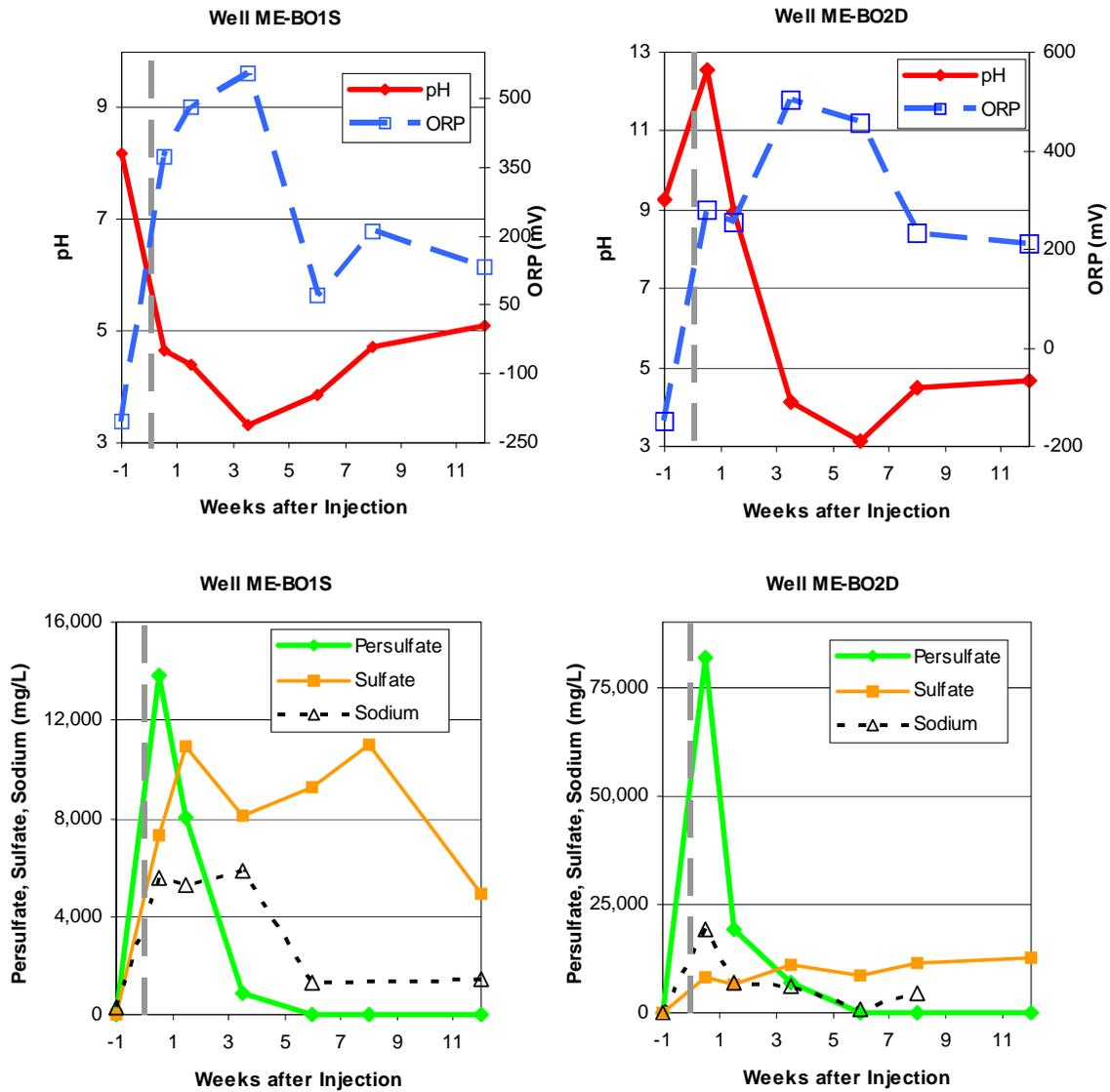
Figure 3. Temporal Summary of Water Quality and Field Screening Parameters Monitoring in Area B Monitoring Wells: ME-BO1S and ME-BO2D.
