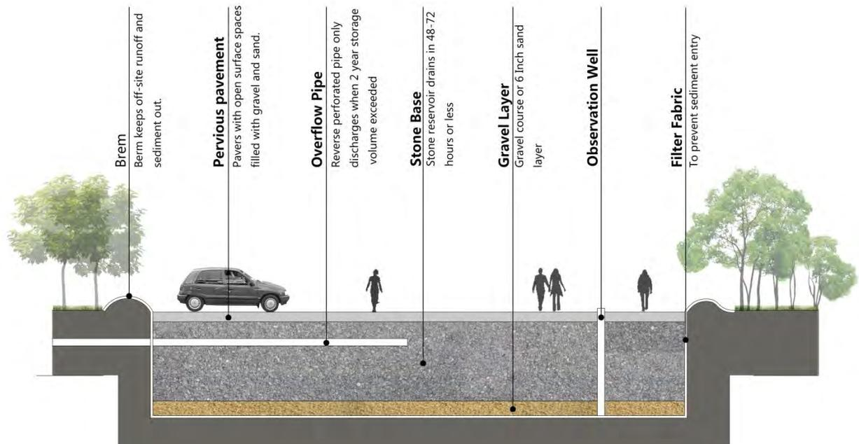
**Figure 8. Structure of permeable pavement**
