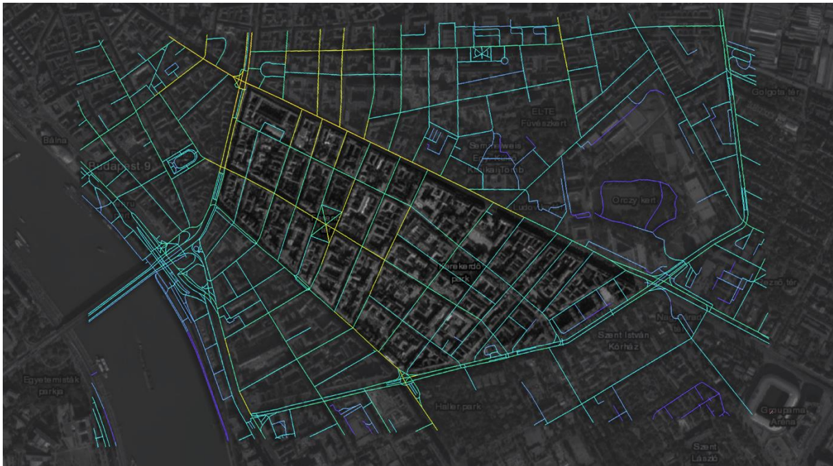
Figure 3. Global integration analysis of IX District of Budapest (1990); performed on DephtmapX– by author
