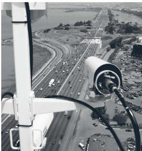
Figure 1.1 A camera installed on top of Pacific Park Plaza recording vehicle trajectory data FHWA (2006a)
