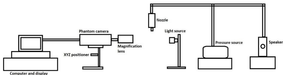
**Figure 2.1:** A schematic of the jetting setup and data acquisition system used in the experiments
