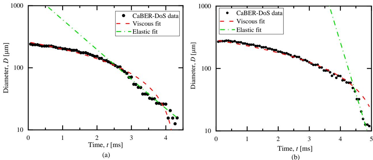
**Figure 3.7:** CaBER-DoS data and curve fits for 16 wt% Vinnol E15 with (a) 0 wt% SiO<sub>2</sub>
