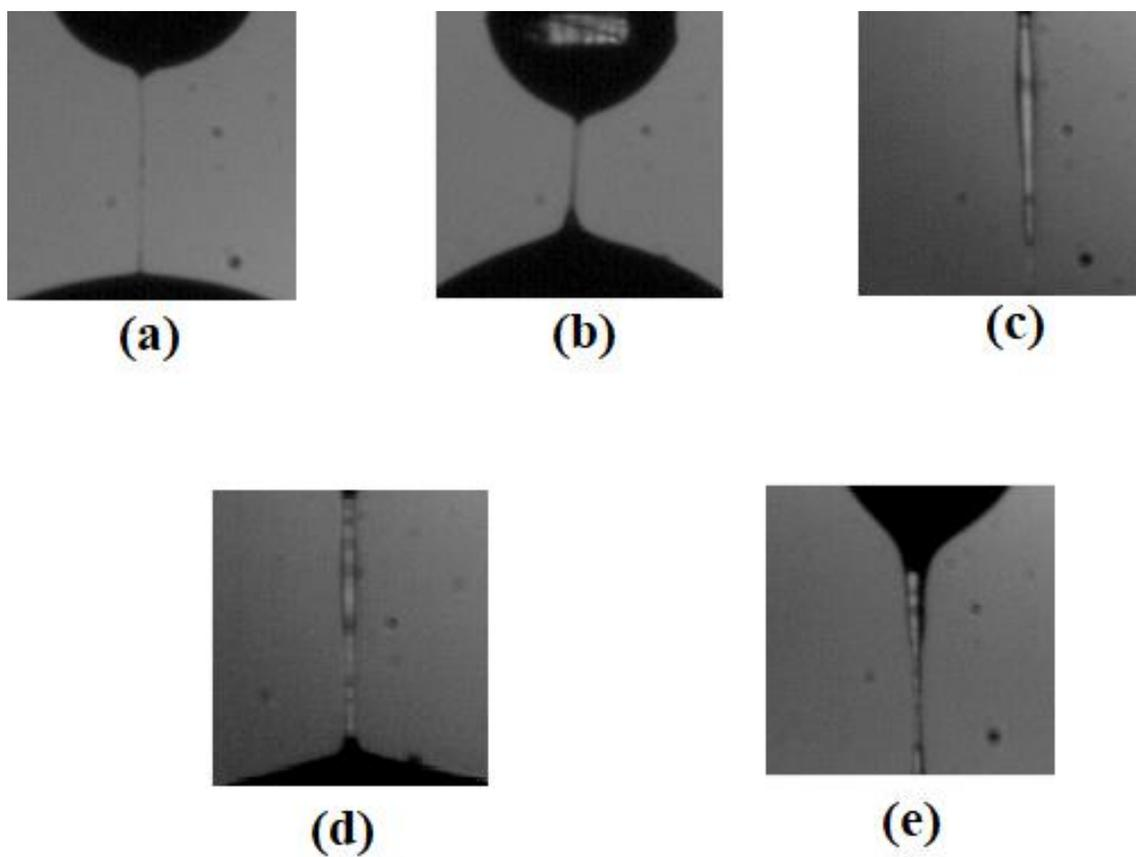
**Figure 3.6:** CaBER-DoS breakup images for 16 wt% Vinnol E15 with (a) 0 wt% SiO<sub>2</sub> (b) 0.5 wt% SiO<sub>2</sub> (c) 1 wt% SiO<sub>2</sub> (d) 2 wt% SiO<sub>2</sub> (e) 4 wt% SiO<sub>2</sub>
