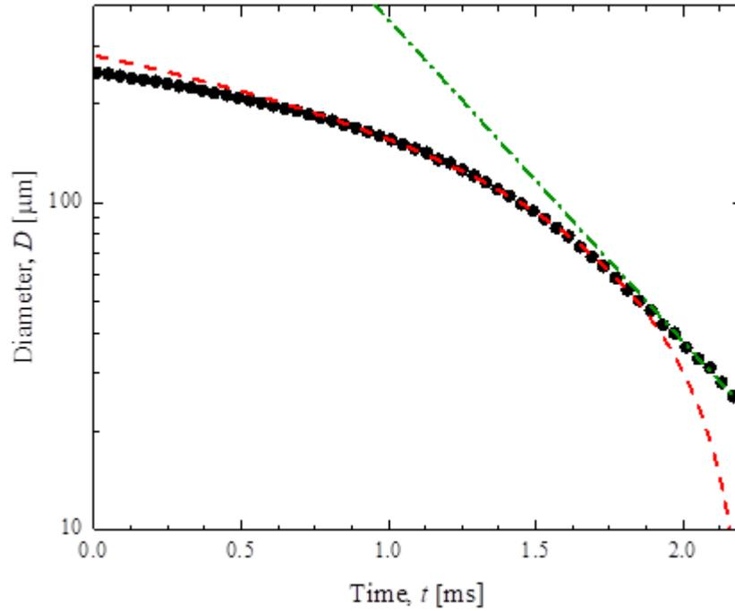
**Figure 2.4:** Sample diameter decay using CaBER-DoS versus time for a weakly elastic fluid with two fits: viscous (- -), fitted using Equation 2 and elastic (- · -), fitted using Equation 3.<sup>35</sup>
