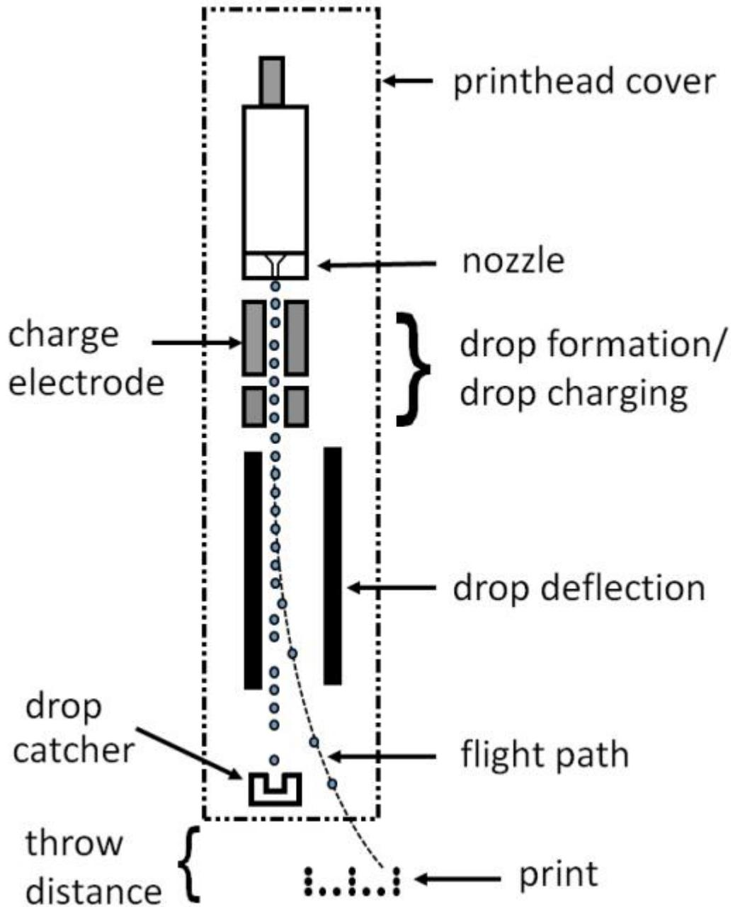
**Figure 1.1:** Sample Continuous InkJet Printing setup.<sup>13</sup>
