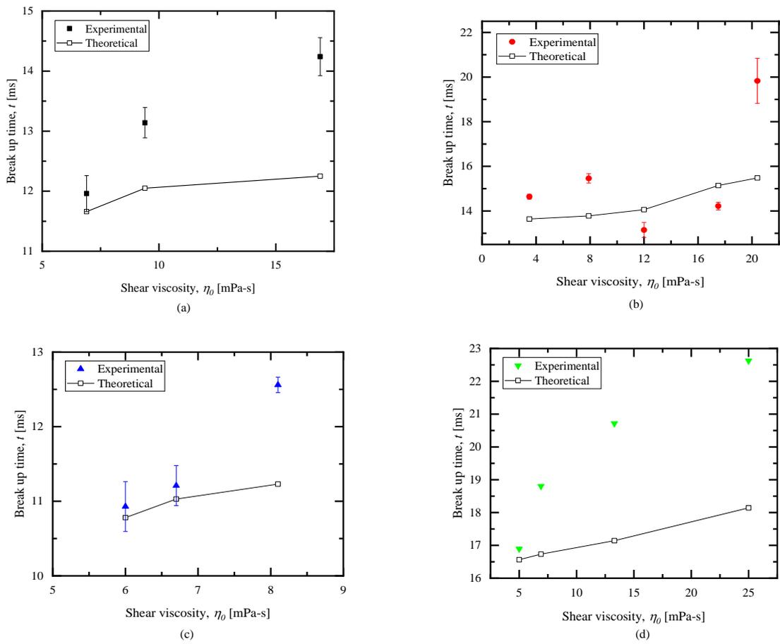
**Figure 3.5:** Theoretical breakup time and experimental results versus shear viscosity for (a) CAB (b) Vinnol E15, (c) Vinnol E22 and (d) Paraloid B66. The theoretical data is represented by hollow squares and lines whereas the experimental data is represented by data points.
