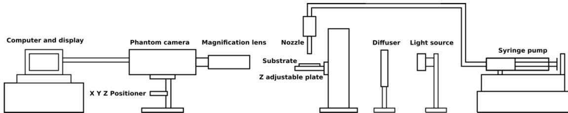
**Figure 2.3:** A schematic of a CaBER-DoS setup and data acquisition system
