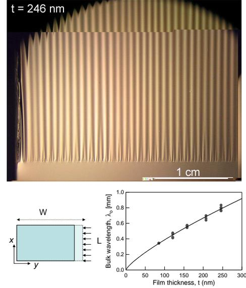
FIG. 1: (A) Image of a wrinkled PS sheet floating on the surface of water, compressed along its length between two razor blades. (B) Sketch of geometry. (C) Bulk wavelength of wrinkles,  $\lambda = 2\pi/q_o$  as a function of film thickness,  $t$ . The solid line is a fit to  $t^{3/4}$ , showing agreement with the prediction of  $q_o = (\rho g/B)^{1/4}$
