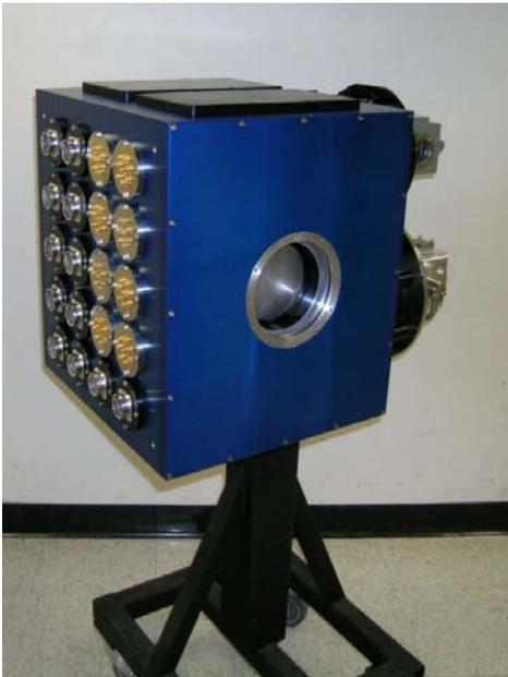
Figure 8: The *SuperCam* cryostat
