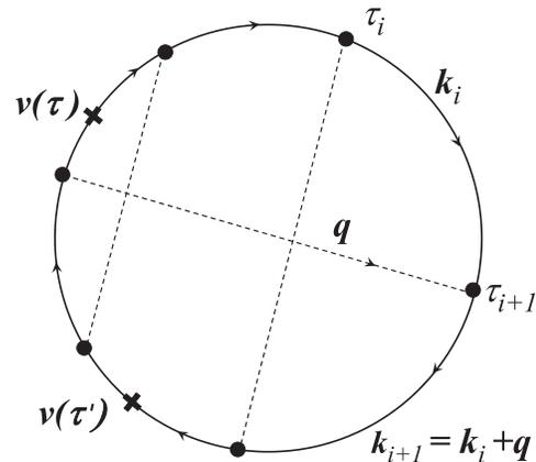
FIG. 1. A typical Feynman diagram contributing to the current-current correlation function. Solid (dashed) lines stand for electron (phonon) propagators  $G$  ( $D$ ), dots represent interaction vertices  $|V\rangle$ , and crosses mark velocity vertices.
