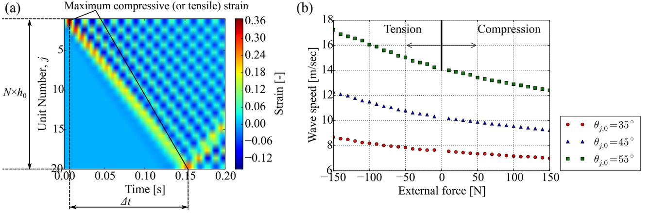
FIG. 5: (Color online) **(a)** Surface map of strain field to calculate wave speed. **(b)** Wave speed of strain waves as a function of external force ranging from  $-150$  N to  $+150$  N. Numerical simulations are based on  $L = 25$  mm,  $m_j = 19.7$  g,  $N = 20$  and  $k_\theta = 1.0$  Nm/rad.
