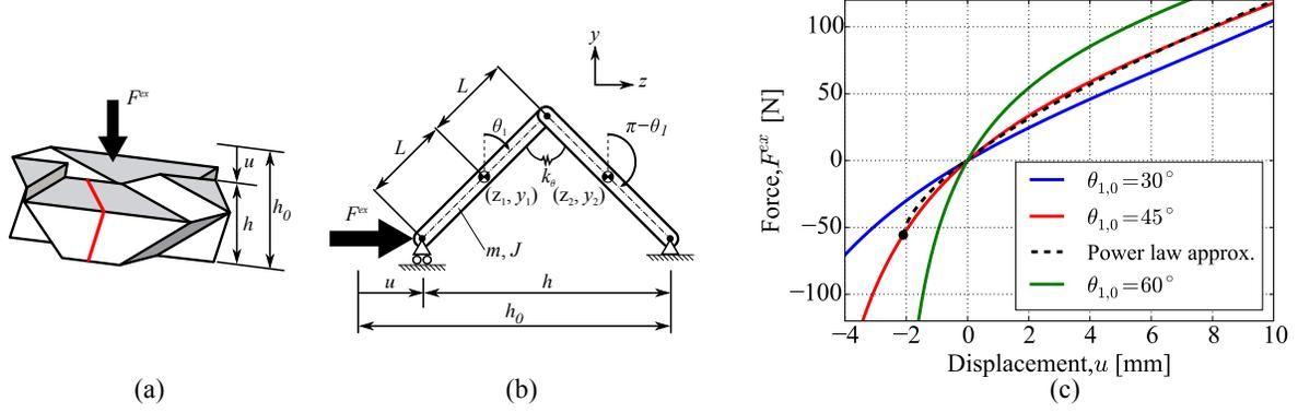
FIG. 2: (Color online) **(a)** TMP unit cell. **(b)** Two-bar linkage model representing the folding motion of the two facets as marked in red lines in **(a)**. **(c)** Force-displacement relationship of the TMP unit cell with  $L = 5$  mm,  $k_\theta = 1.0$  Nm/rad, and different initial folding angles:  $\theta_{1,0} = 30^\circ$ ,  $45^\circ$ , and  $60^\circ$ . Dashed line indicates a power law approximation of  $\theta_{1,0} = 45^\circ$  case.
