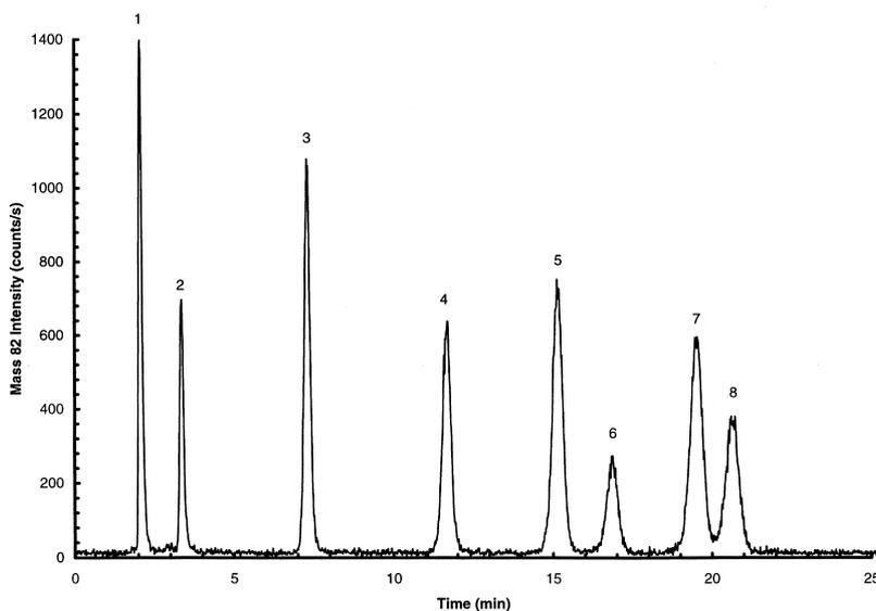
Fig. 5. Ion pair chromatogram of selenoamino acid standards; approximately 300 ppb Se each. Mobile-phase flow-rate, 1.0 ml/min. Peaks: 1, selenocystine; 2, Se-methyl-DL-selenocysteine; 3, selenomethionine; 4, Se-allyl-DL-selenocysteine; 5, *cis*-Se-1-propenyl-DL-selenocysteine; 6, *trans*-Se-1-propenyl-DL-selenocysteine; 7, selenoethionine; 8, Se-propyl-DL-selenocysteine.
