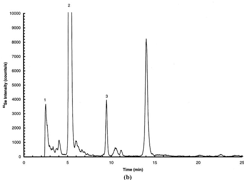
Fig. 6. (a) Ion pair chromatogram of 1355-ppm Se-garlic extract diluted 1:1 with water. Mobile-phase flow-rate, 0.6 ml/min until 6 min, then 1.0 ml/min. UV absorbance monitored at 254 nm. (b) Selenium 82 chromatogram for same sample injection shown in (a). Peaks: 1, inorganic selenium; 2, Se-methyl-DL-selenocysteine; 3, selenomethionine. Maximum intensity of Se-methyl-DL-selenocysteine peak was 110 000 counts/s.
