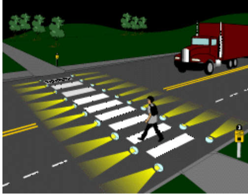
Figure 2 In-Pavement Warning Lights System (5).
