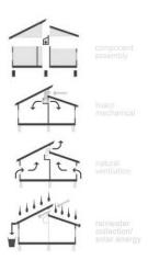
The design was to offset the roofline so in order to vent hot air during the summer, passively cooling the compact house scheme. Underneath the clerestory, the ductwork is integrated into the wall cabinets to further insulate and centralize the output. The design allows for the minimal length of ductwork to feed both vertical halves of the floor plan. The two base modules in plan also sit offset from each other.
