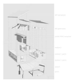
The SIPs are used for the exterior walls, raised flooring and pitched roofs that are angled. An important design aspect was to create the greatest height allowable through the careful study of the slopes. The slopes were determined by transport limits, the diagonal being the maximum length in the transport volume. Normally in manufactured housing, the roof lines and interior spaces are compromised by the limit in height achievable during transport.
