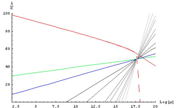
FIG. 6: The evolution of coupling constants with higher order groups up to  $SU(113)$  (solid red line) and  $SU(7919)$  (dashed red line) given  $U(1)$  hypercharge. Higher order coupling constants are shown in grayscale
