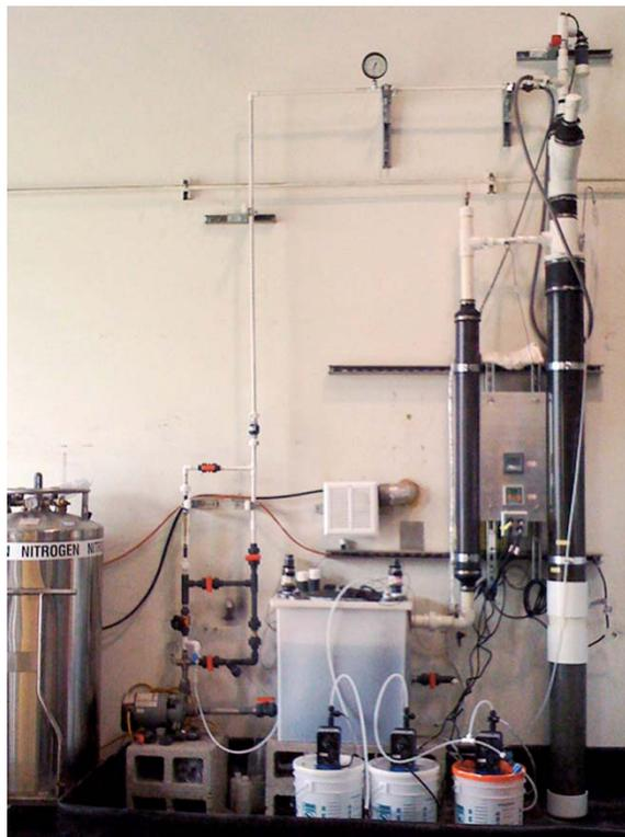
Figure 1. Anaerobic fine media fluidized bed bioreactor system.
