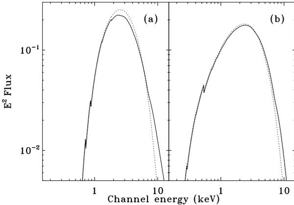
**Figure 2.** The effects of the Comptonization in LMC X-1 (a) and in LMC X-3 (b). Solid line: spherical CMCD model with the best fit parameters; dotted line: CMCD model with the same parameters but  $\tau=0$ , which is equivalent to the MCD model.
