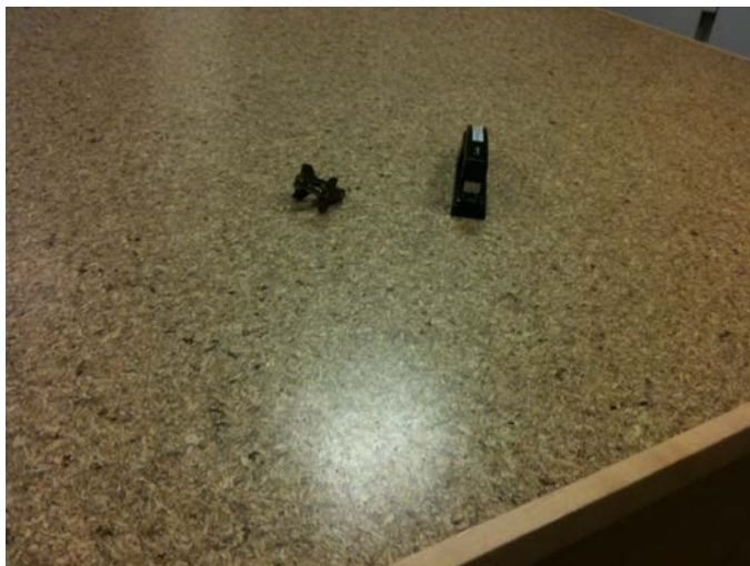
A plan table made from recycled and crushed sunflower seeds. Source: M. Larossi
