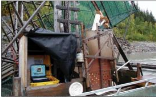
This video system continuously records fish passing through the fishwheel and captures the information on a laptop for later analysis.
