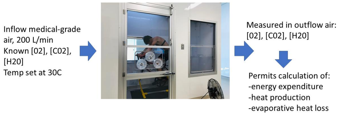
Figure 4: Schematic of flow-through respirometry using the University of Massachusetts Human Testing Center’s flex room calorimeter.
