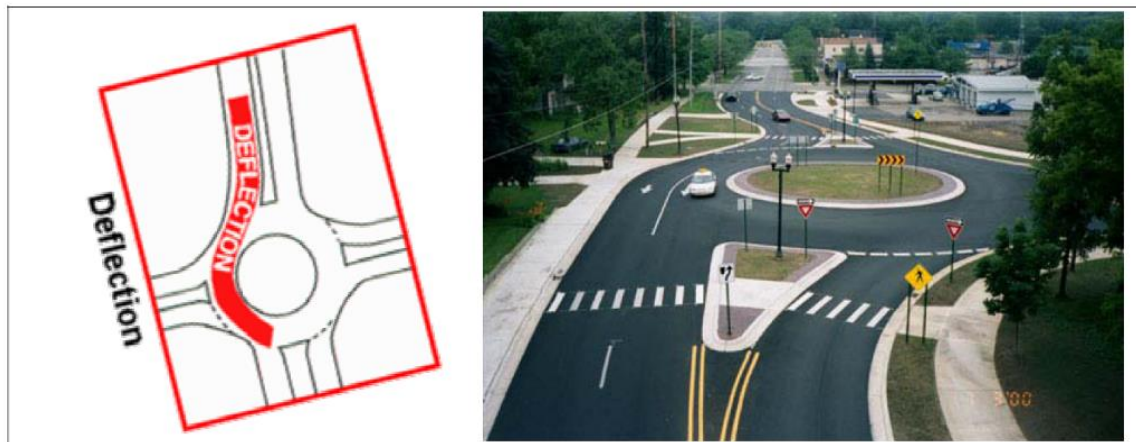
Figure 4: Deflection angle in a roundabout
