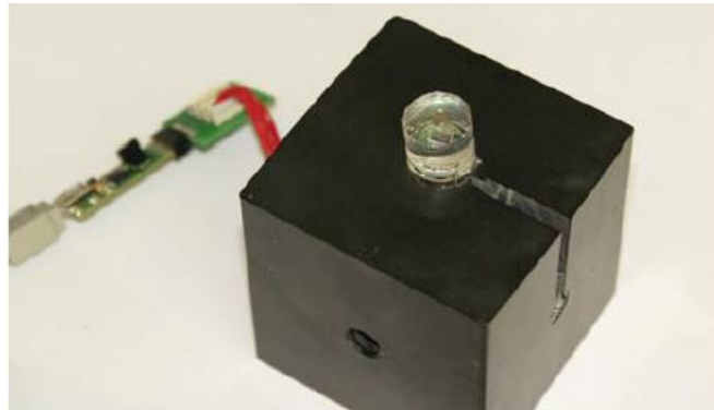
Figure 2.7: Tactile sensor based on one 3D Hall sensor (27)
