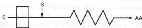
Fig. 1. Single line manifold. C is a distilled water carrier stream, S is the sample injection valve and AA is the model 5000 spectrometer. The connection between the valve and the detector was the minimum length of tubing possible.
