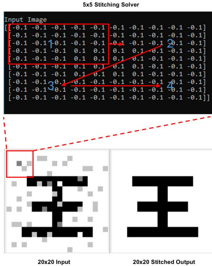
Figure 2.5: Proposed stitching solver to process a larger image (20×20) on a smaller CeNN (5×5).
