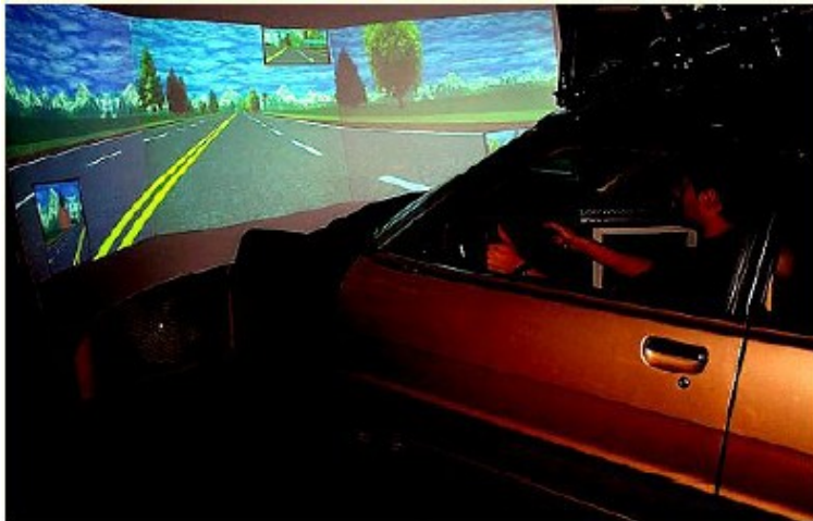
Figure 7. Configurations for DATS (Allen et al., 2003). (a) Single-monitor system. (b) Three-monitor, wide field of view system. (c) Cab system with curved projection screen.
