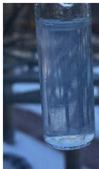
Figure 20 Collagen fibers formed on dialysis into Tris HCl
