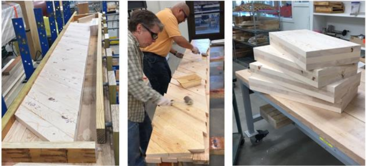
Figure 4.1: The size of the three layers short-span CLT panel for different board orientation
