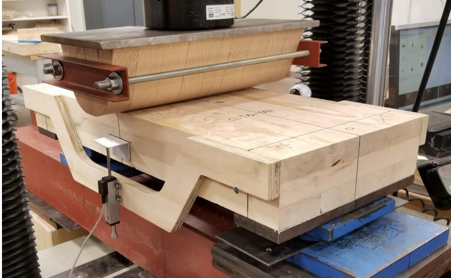
Figure 4.4: Typical test setup for short-span CLT test
