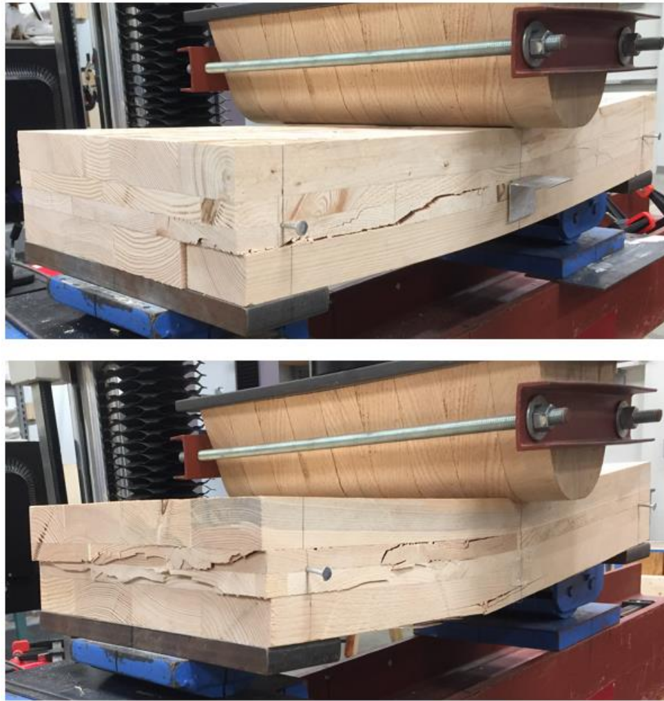
Figure 5.5: Typical failure of short-span asymmetric panels: 45^\circ CLT (top) 30^\circ CLT (bottom)
