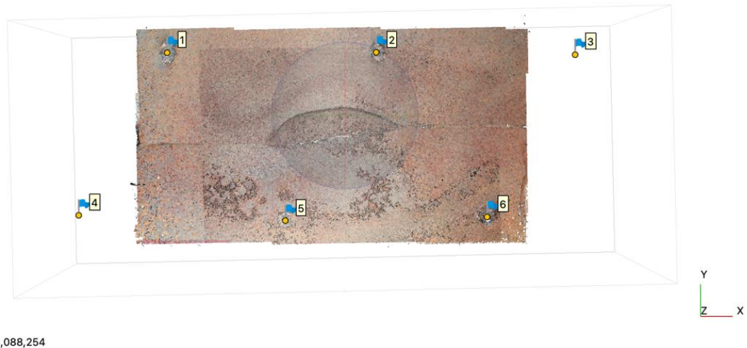
Figure 1.4: Final dense point cloud with over 4 million data points generated in Metashape. The blue flags and numbers indicate the position of the six control points placed on top of the surface of the clay. We cropped the raw dense point cloud to only show the area of interest. This dense point cloud represents the final stage of a 15° and 2 cm stepover restraining bend experiment.
