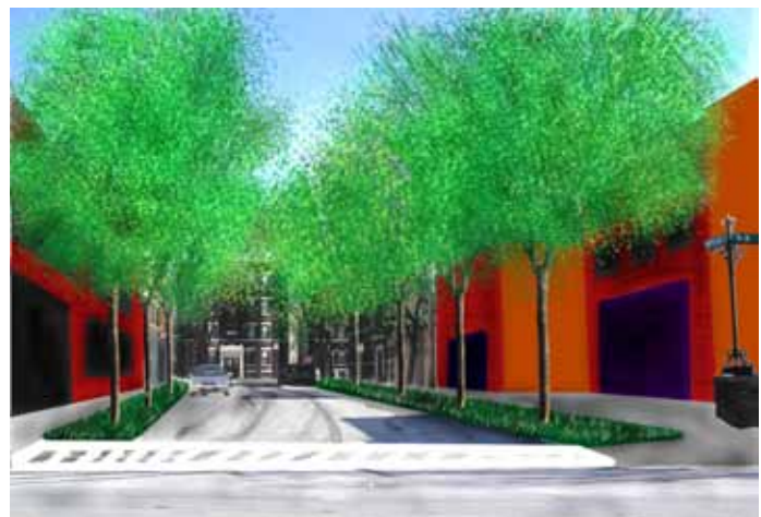
Dwight St. Extension becomes a planted boulevard. Median strips and street edges accommodate swales, collecting runoff from the streets.
