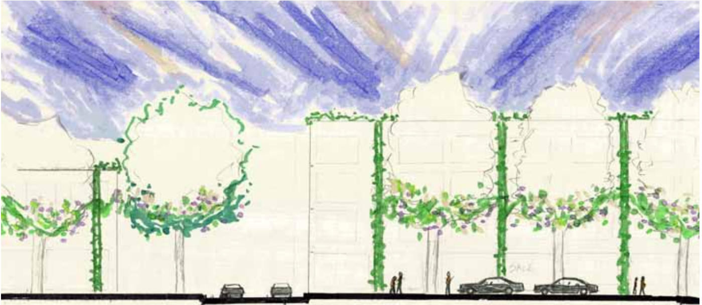
Vegitated vertical infiltration Swales are located on either side of Main Street. They capture Roof runoff which is stored in underground Systems.
