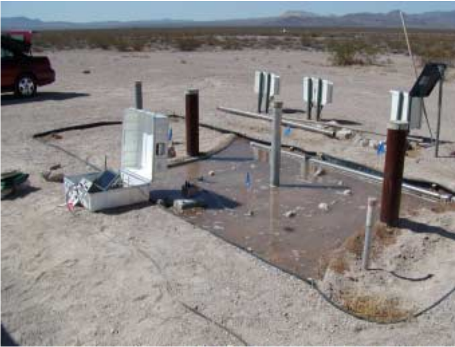
Figure 3. INL wireless sensor platform field test. For this test, the buried sensor packages (marked by the blue flags) are located on the exterior of the antenna encircling the aluminum well casing.
