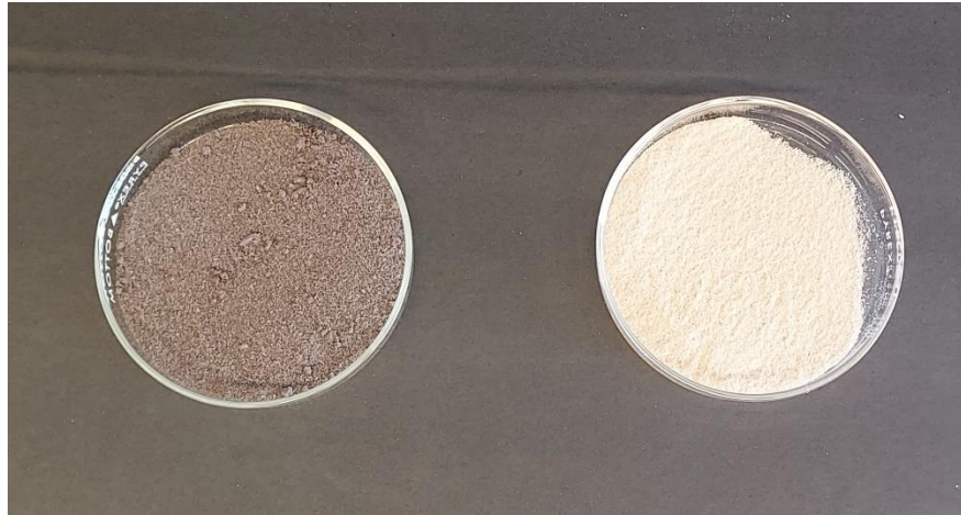
Figure 2.2: A photo of treated sawdust mixture, or bioCap (left), next to untreated sawdust (right).
