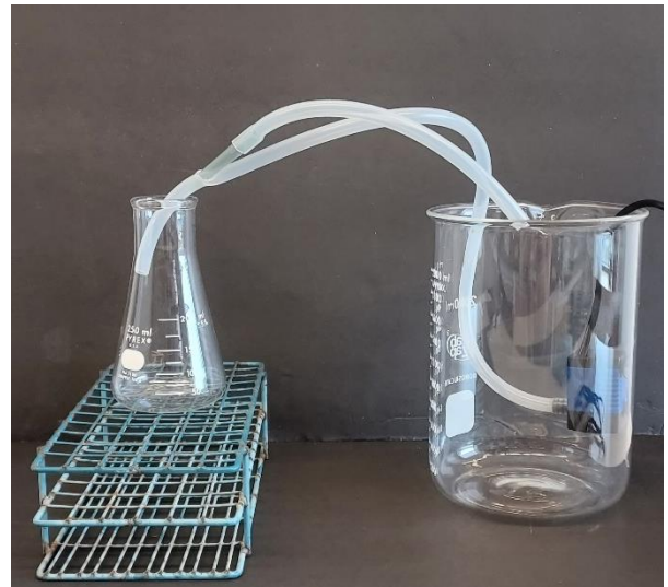
Figure 2.3: A photo of fish pump preparation, demonstrating the siphoned tubing feeding back into the solution.
